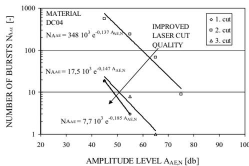
Fig. 9. Amplitude distribution of AE burst signals in laser cutting of mud-guard.
