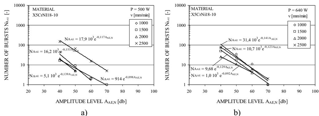
Fig. 7. Amplitude distribution of AE burst signals after laser cutting of austenitic stainless steel under different conditions: a)  $P = 500$  W, b)  $P = 640$  W.
