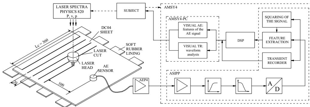
Fig. 1. AE capture during and after laser cutting of flat sheet.
