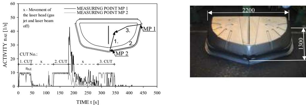
Fig. 8. Activity  $n_{AE}$  of AE signals during and after cutting operations in laser cutting of deep-drawn part.
