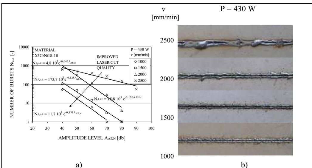
Fig. 6. a) Number of AE bursts  $N_{AAE}$  above selected amplitude levels of AE signals  $A_{AE,N}$  immediately after termination of laser cutting of sheet X5CrNi18-10 with power  $P = 430$  W and b) images of dross at lower cut edge.
