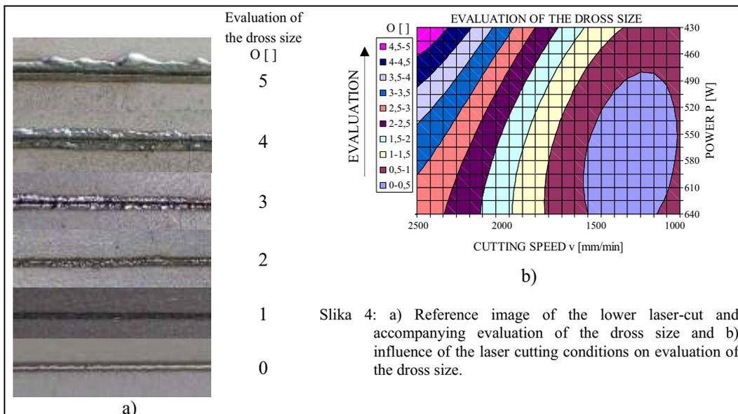
Slika 4: a) Reference image of the lower laser-cut and accompanying evaluation of the dross size and b) influence of the laser cutting conditions on evaluation of the dross size.
