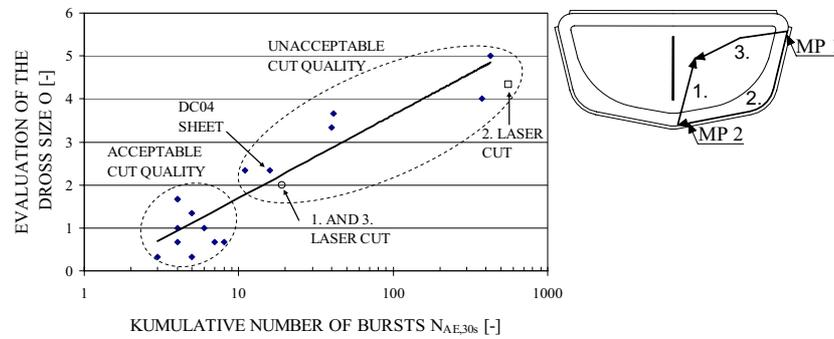
Fig. 5. Dependence between number of AE bursts  $N_{AE,30s}$  and evaluation of dross size  $O$ .
