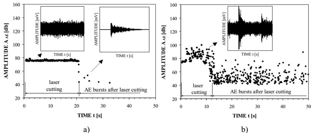
Fig. 2. Acoustic emission during and after laser cutting of DC04 steel sheet under two laser cutting conditions: a)  $P = 430 \text{ W}$ ,  $v = 1000 \text{ mm/min}$  and b)  $P = 430 \text{ W}$ ,  $v = 2500 \text{ mm/min}$ .
