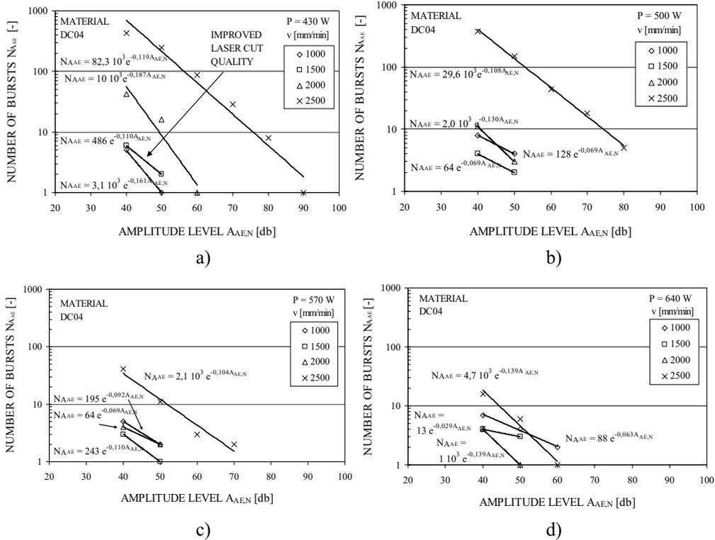
Fig. 3. Number of AE bursts  $N_{AAE}$  above various AE signal amplitude levels  $A_{AE,N}$  after laser cutting with different powers: a)  $P = 430$  W, b)  $P = 500$  W, c)  $P = 570$  W, d)  $P = 640$  W.
