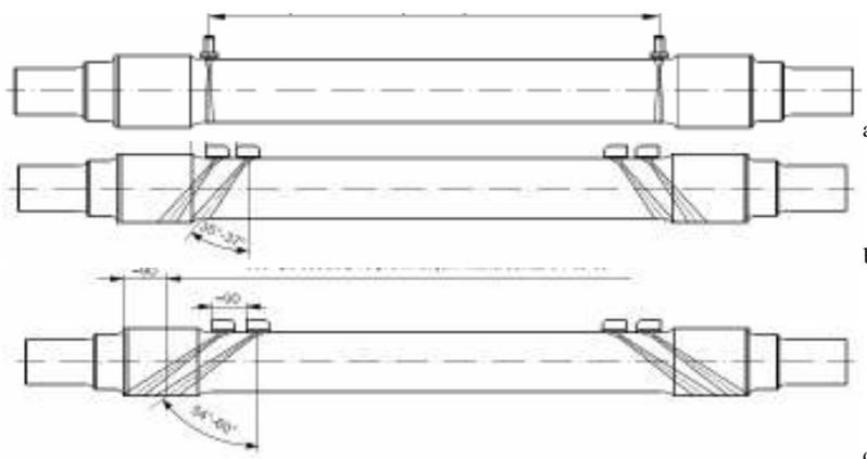
**Figure 4. Ultrasonic testing of axles with normal probe (a), 37° angle probe (b), and 60° angle probe (c)**
