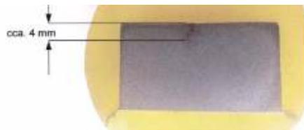
**Figure 11. Depth of transverse crack in axle shown in macro section.**
