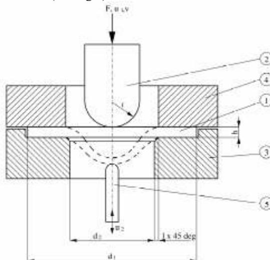
Fig.4 Cross-sectional scheme of the testing apparatus (1-specimen, 2-punch, 3-lower die, 4-upper die, 5-deflection measurement rod), [6].
