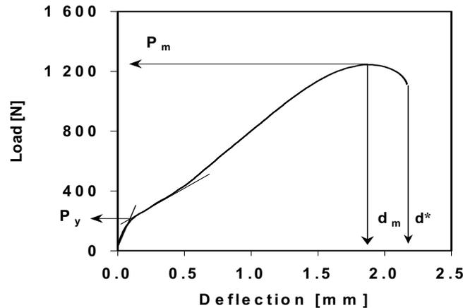
Fig. 5 Load displacement curve
