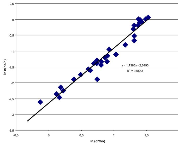
Fig. 9 Relationship between  $\ln(h_0/h_f)$  and  $\ln(d^*/h_0)$  for the CrMoV rotor steel [13]
