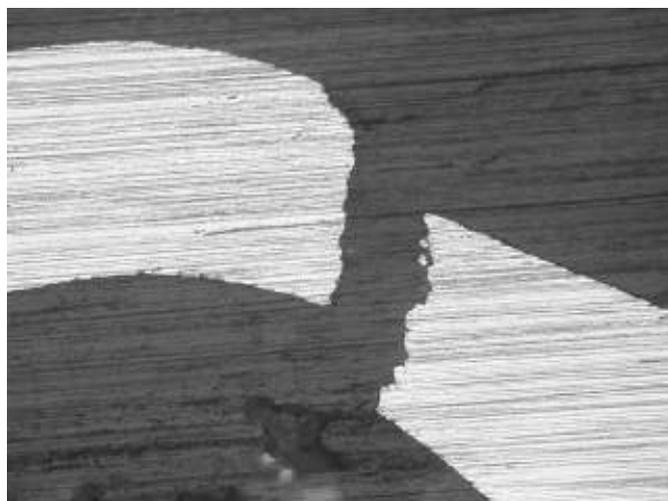
Fig.10 Metallographic sample of failed SP test specimen tested at  $-160^{\circ}\text{C}$ , [13]
