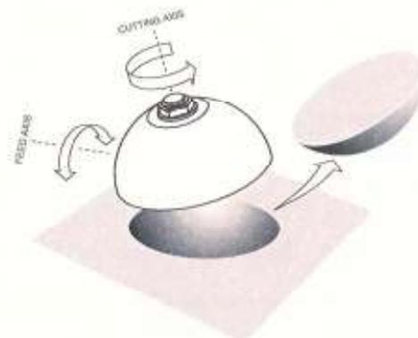
Fig.2 The principle of the sampling by SSam<sup>TM</sup>-2
