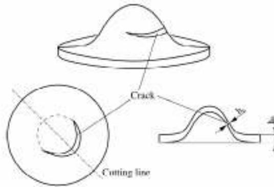
Fig.8 Procedure for determination of effective fracture strain  $\epsilon_f$ , [6].
