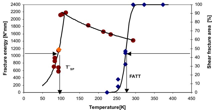
Fig.6 Transition behaviour observed in SP tests and impact bend tests results.
