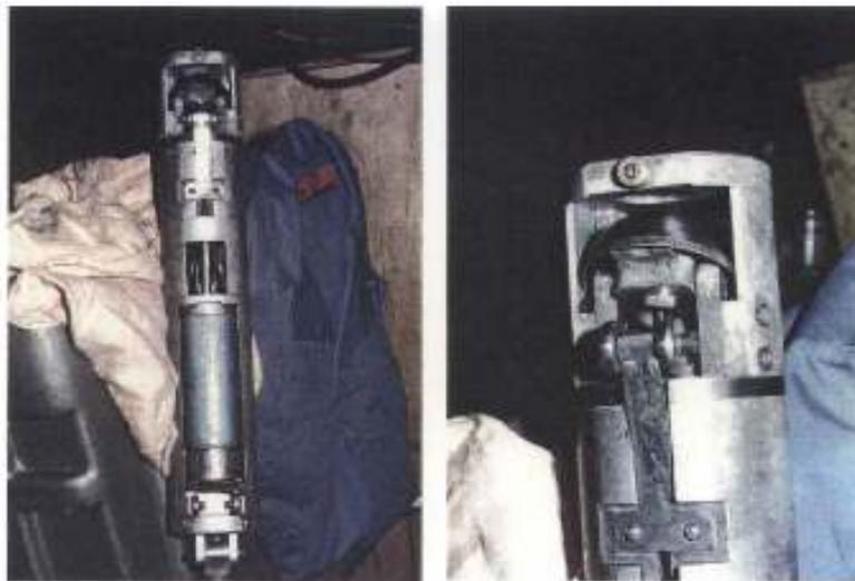
Fig.1 Rolls-Royce SSam<sup>TM</sup> – 2 scoop sampling machine, [6]
