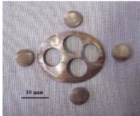
Fig. 3 Example of a miniature sample removed with the scoop system with SP test specimen blanks subsequently machined [6].
