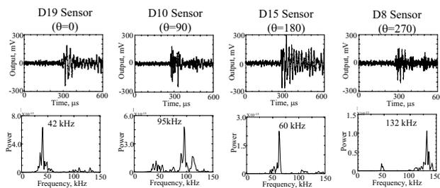
Fig.3 Waveforms and frequency spectra of AE signals detected by ITFDS
