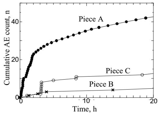
Fig.18 Cumulative AE counts from three rust pieces
