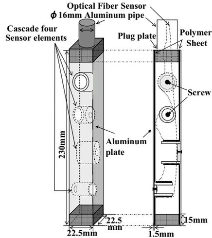
Fig.1 Immersion type four direction AE sensor using optical fiber
