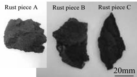
Fig.16 Three rust pieces to monitor liquid borne AE
