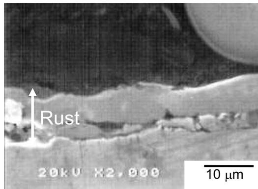
Fig.14 Cross section of bare steel plate exposed to mist spray corrosion after 15 days
