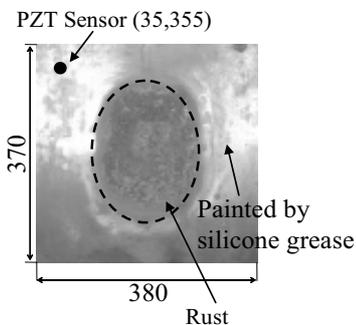
Fig.7 Sample A with rust before the corrosion test
