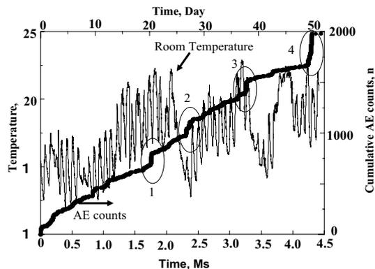
Fig.8 Change of Temperature and cumulative AE counts by optical fiber AE system
