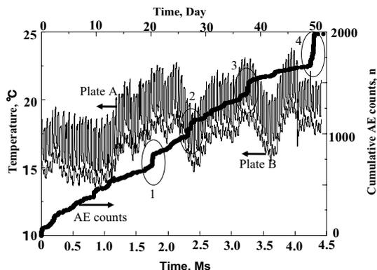
Fig.9 Change of Temperature of plate A and B and cumulative AE counts by optical fiber AE system
