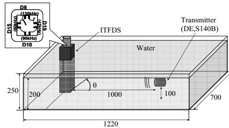
Fig.2 Experimental setup to study the directivity of the ITFDS
