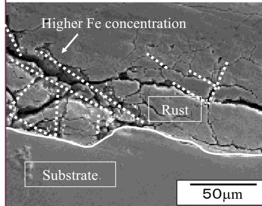
Fig.15 Transverse SEM of rust on sample B exposed to corrosion acceleration test
