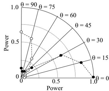
Fig.5 Amplitude profile as a function of the angle  $\theta$  of ITFDS
