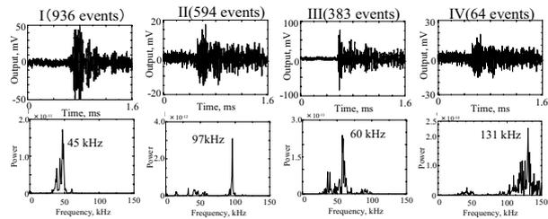
Fig.10 Waveforms and their frequency spectra detected by four optical fiber sensors
