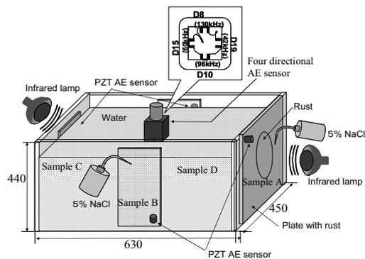
Fig.6 Experimental setup for monitoring AE from rust fracture on corroded four plates
