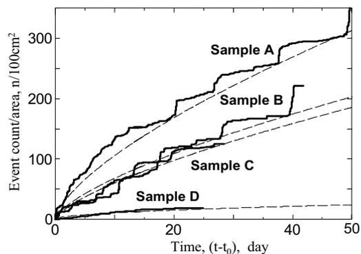
Fig.12 Change of classified event counts of AE signals from four samples
