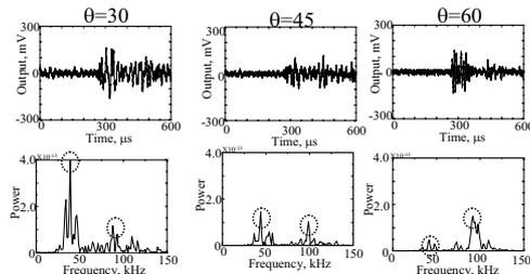
Fig.4 Waveforms and frequency spectra of water born AEs detected by ITFDS at  $\theta = 30, 45$  and  $60$
