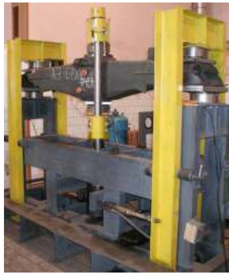
Fig.7. AE installation for freight-car truck cast details diagnostics (solebars and bogie bolster)
