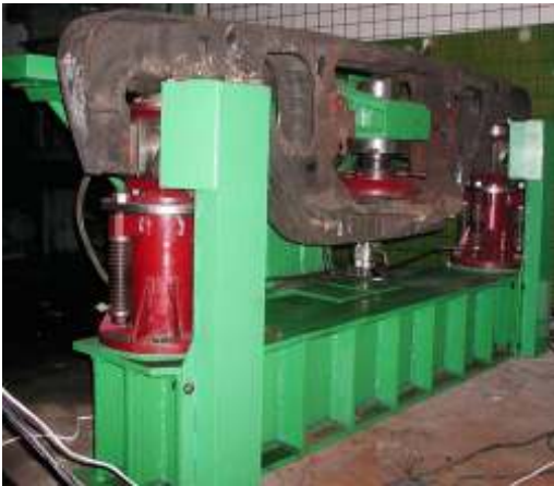
Fig.7. AE installation for freight-car truck cast details diagnostics (solebars and bogie bolster)
