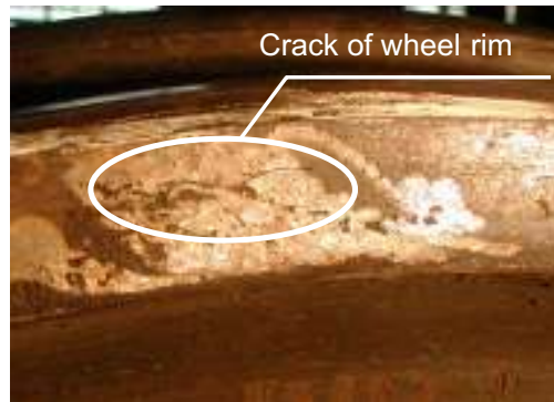
Fig.6. The defects detected in wheelset pairs using AE diagnostics
