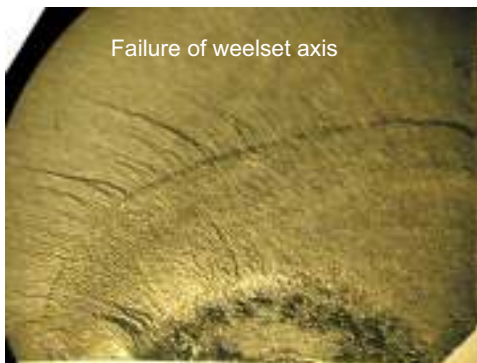
Fig.6. The defects detected in wheelset pairs using AE diagnostics
