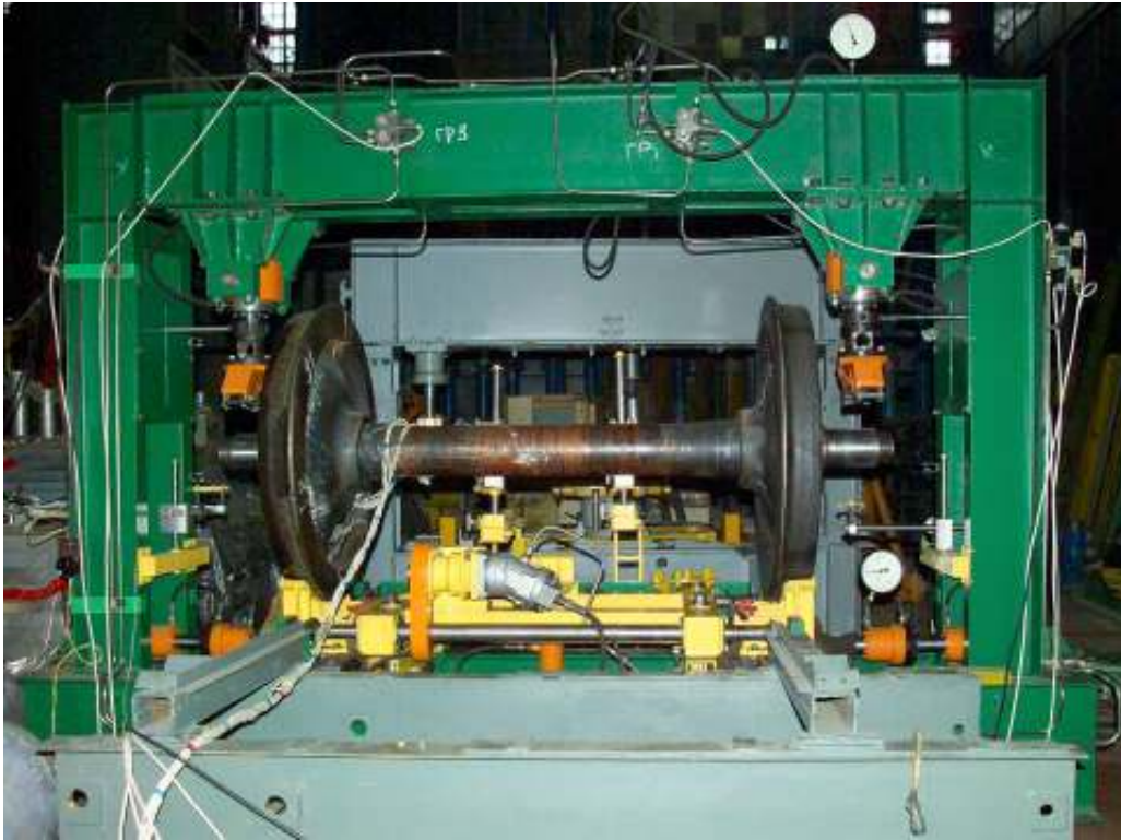
Fig.5. AE installation for wheelset pairs diagnostics
