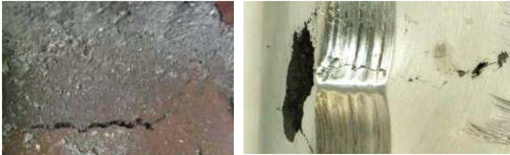
Fig.8. The defects detected in basic surface of bogie bolster using AE diagnostics
