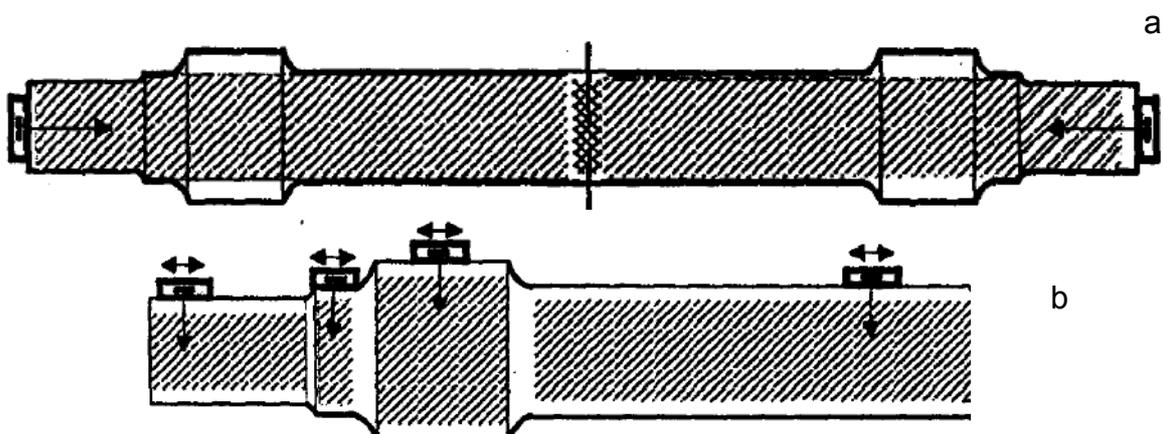
Fig.1. The schemes of ultrasonic through transmission method of wheelset axle testing: a – longitudinal sounding from the face of Wheelset Axle, b – radial sounding from lateral surface.
