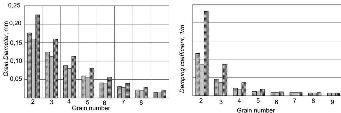
Fig.3. Variations in grain sizes (a) and damping coefficients (b) for different grain numbers
