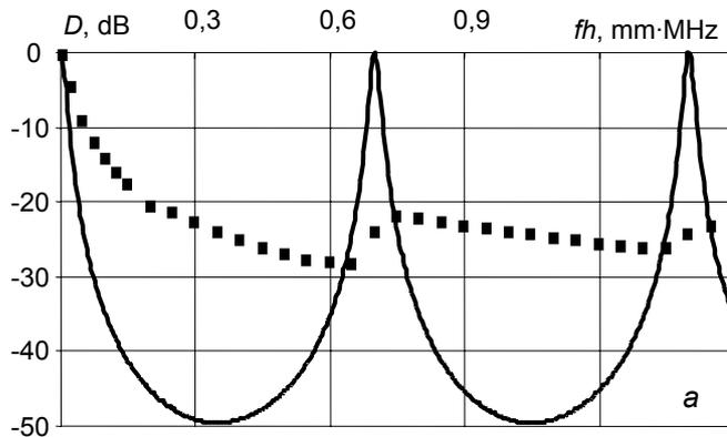
Fig.2. Transparency coefficient  $D$  for the cases of uniform (—) and non-uniform (- - -) thickness contact layer
