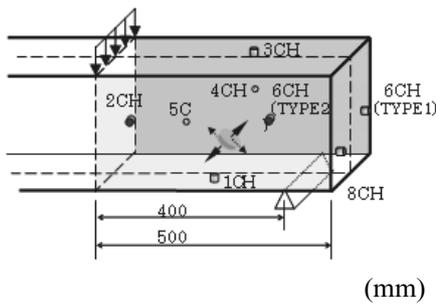
Fig. 5 AE sensor array.
