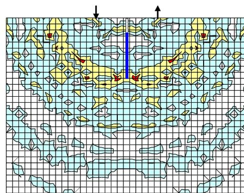
Fig. 10 SIBIE analysis in an open crack.
