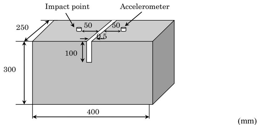
Fig. 9 Specimen with a surface crack.
