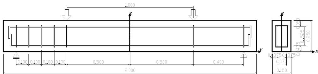
Fig. 4 Sketch of RC specimen (unit:m)
