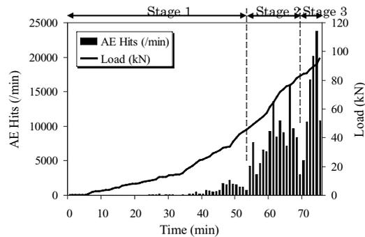
Fig. 6 AE generating behavior under bending
