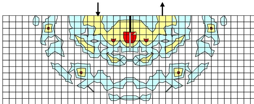
Fig. 12 SIBIE analysis in an improperly repaired crack.
