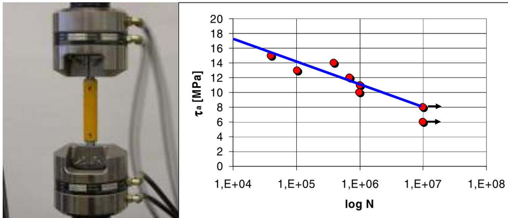
Fig. 16 & 17 Fatigue testing of glued joint of G/E composite tubes and S-N curve of the joint
