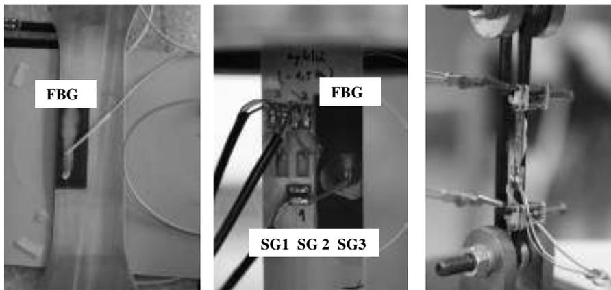
Figures 21 & 22 Application of the strain gauge (SG) and fibre Bragg gratin sensors (FBG)
