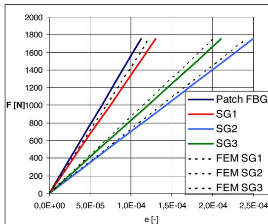
Figures 21 Comparison of the FEM, Strain gauge and FBG sensors strain signal measurement in different places on the carbon patch
