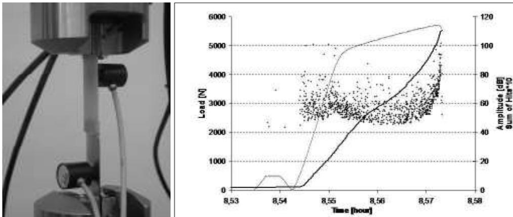
Fig. 19 Acoustic emission monitoring of bonded joint
