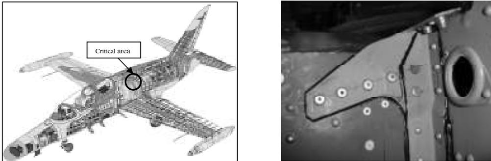
Fig. 1 & 2. Aircraft L159A and detail of the critical area at auxiliary stringer
