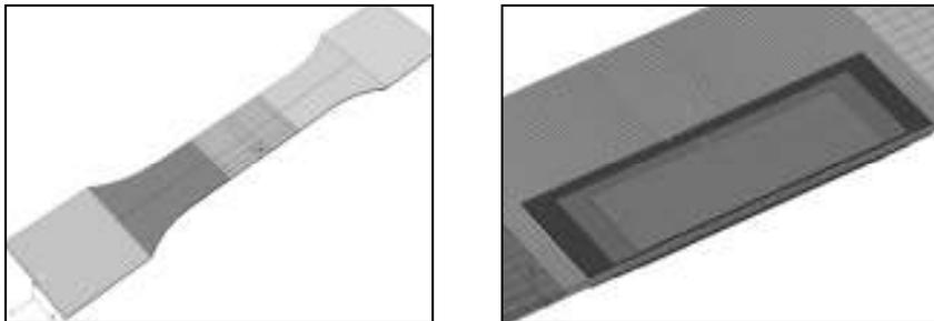
Fig. 7 & 8. The aluminum specimen geometry depicting the asymmetrically cracked/drilled gauge region and the geometry/orientation of the applied composite patch in the CTU FE model.
