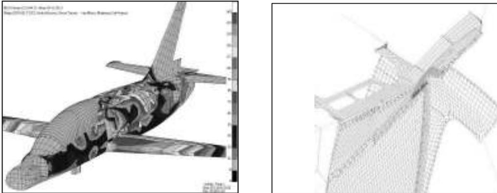
Fig. 5 & 6. A global FE model and FE submodel of the critical area at auxiliary stringer
