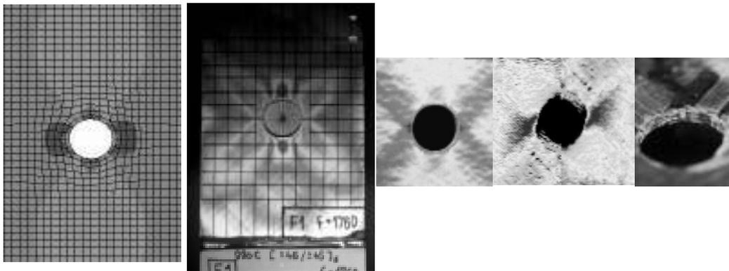
Fig. 18 Comparison of the stress concentration around the hole in axial loaded composite plate: FEM, photostress, ARAMIS, SPATE, strain gauge
