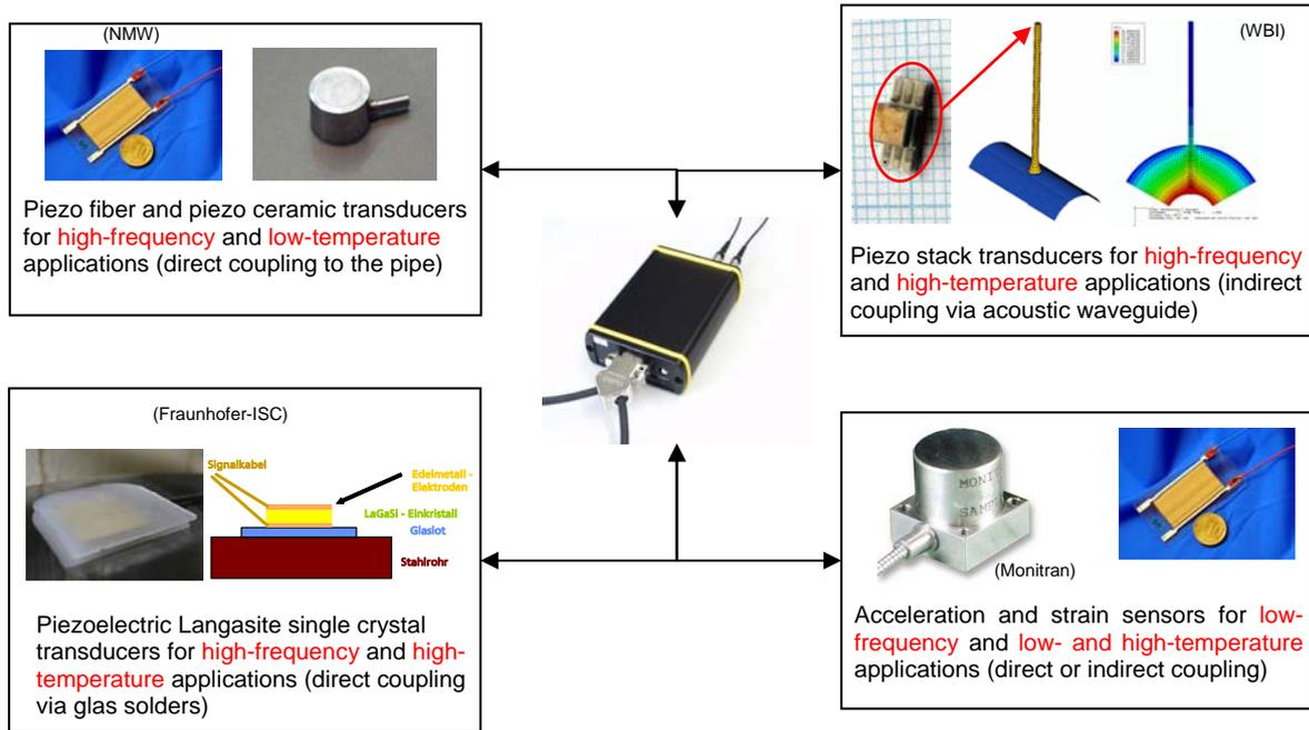
**Figure 13:** Conception of the modular transducer system. The SHM network will be able to manage different kinds of transducers and sensors for low- and high-temperature applications and for low- and high-frequency monitoring.
