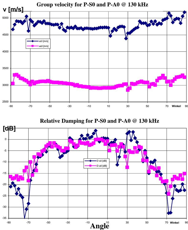
**Figure 6:** Experimental results for angle-dependent group velocity and damping coefficient for P-S0 (dark blue) and P-A0 mode (magenta) at a center frequency of 130 kHz. The group velocities can be seen as roughly constant in each direction. With the exception of large angles  $>70^\circ$  the relative damping coefficients for P-S0 and P-A0 are similar to each other. For the range between  $\pm 50^\circ$  a damping of only 5-10 dB is obtained.
