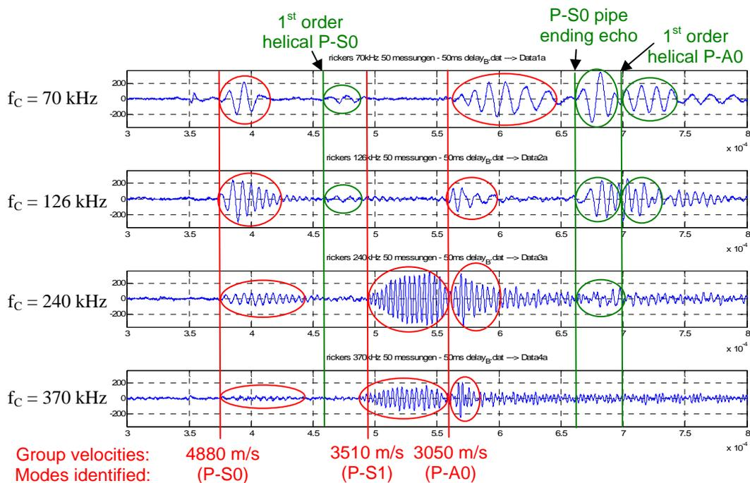
**Figure 4:** Measured time-domain signals along the steel pipe for four different center frequencies of the input pulse. All elementary wave modes as predicted by theoretical and numerical investigations (including helical modes) could be identified.
