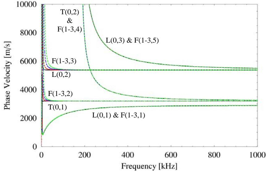
**Figure 1:** Phase velocity as a function of frequency for various guided wave modes in a free steel pipe with a diameter of 406 mm and a wall thickness of 9 mm. The frequency band between 50 and 200 kHz seems to be most appropriate for long-range SHM applications since in this region only a limited number of wave modes is available and can be easily separated if necessary.
