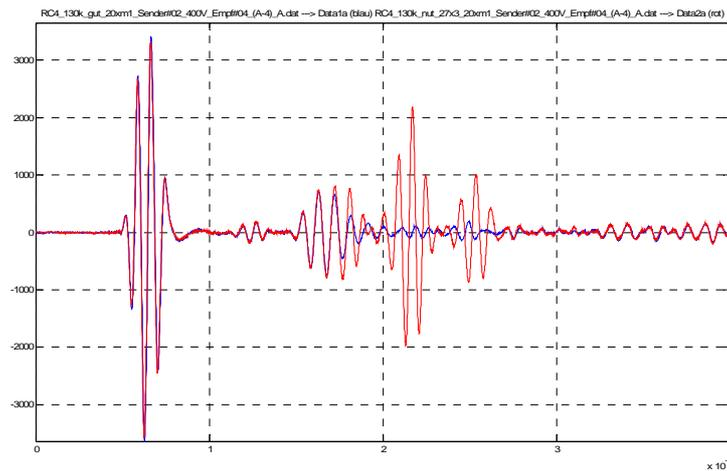
**Figure 9:** Results for three different notches (red curves) using transducer #2 as actuator and #4 as sensor. The blue curve represents the reference measurement (baseline) without notch.
