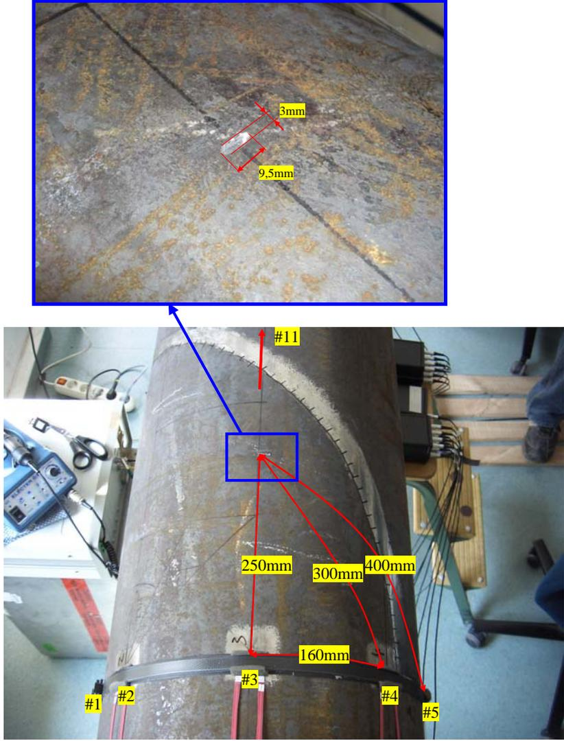
**Figure 8:** Details of the set-up showing the distance of the notch to the relevant transducers. For the measurements shown in the following Fig. 9, transducers #2 and #4 were used.
