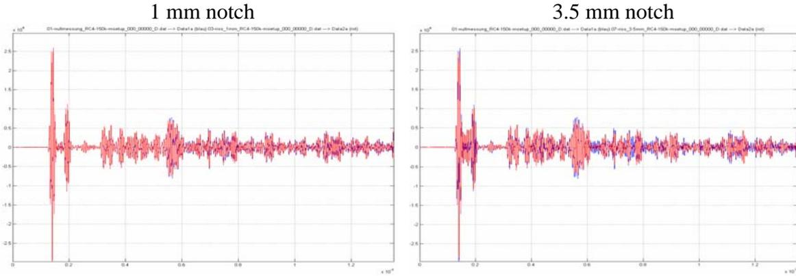
**Figure 11:** Typical guided wave system response of the Titanium elbow along path A-D<sub>1</sub> for the 1 mm and 3.5 mm deep notch, respectively. Red curves: reference state without notch; blue curves: elbow with notch.
