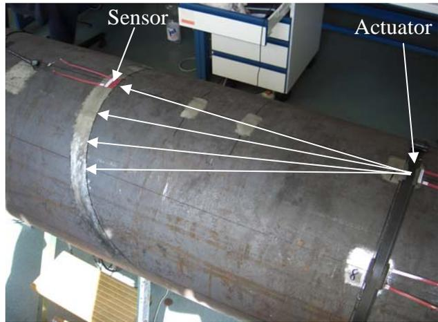
**Figure 5:** Experimental set-up as used for the measurement of the directivity patterns of P-S0 and P-A0 modes generated by a piezo fibre transducer. The sensor on the opposite side was shifted along the curved black line. Each point on the line has the same geometrical distance of 50 cm to the source position.
