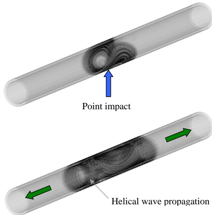
**Figure 2:** Guided elastic wave propagation in a steel pipe generated by a mechanical radial force point impact on the outer surface of the pipe. The wave front pictures were calculated by using the 3-D elastodynamic finite integration technique in cylindrical coordinates (CEFIT [7]) and show the helical nature of the elastic wave field. Further interesting numerical and analytical investigations of guided waves in free pipes can be found in [8, 9].
