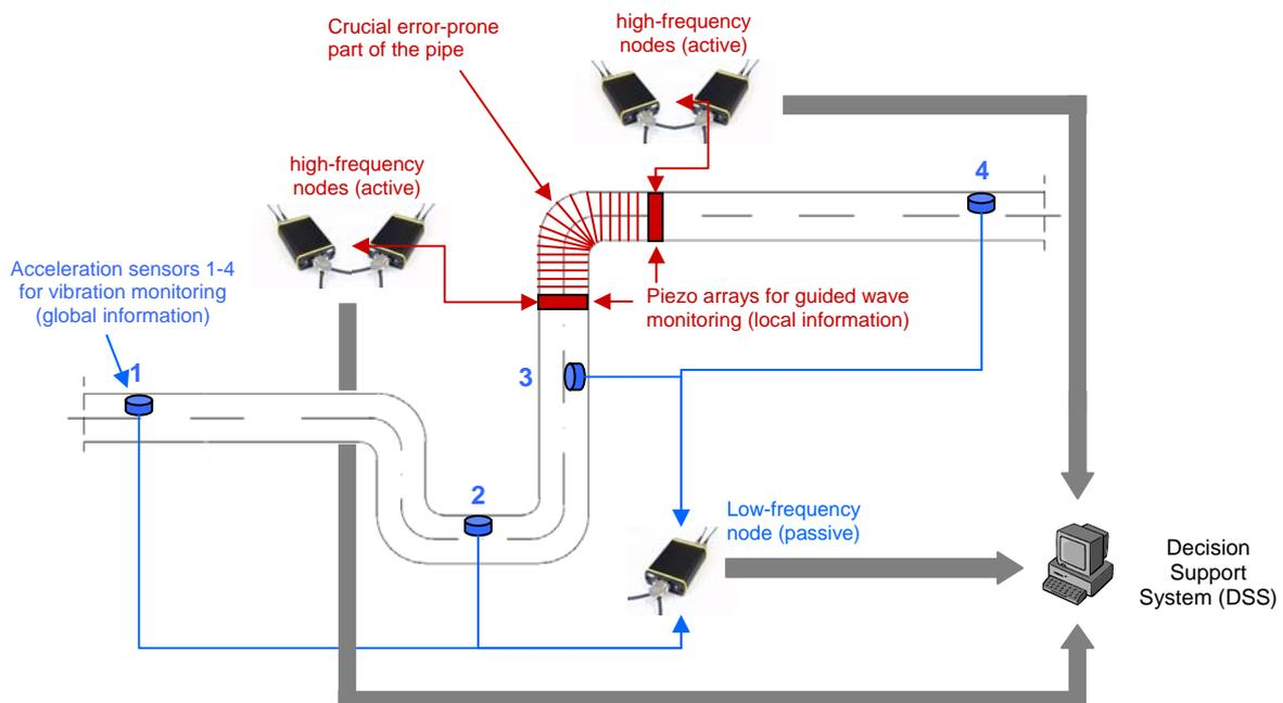
**Figure 14:** Combination of low- and high-frequency monitoring. While the passive low-frequency nodes with acceleration and strain sensors are responsible for global vibration monitoring of the structure (providing information on basic boundary conditions caused by hangers and dampers) the active high-frequency guided wave nodes are used to monitor local crucial and error-prone parts of the piping system.
