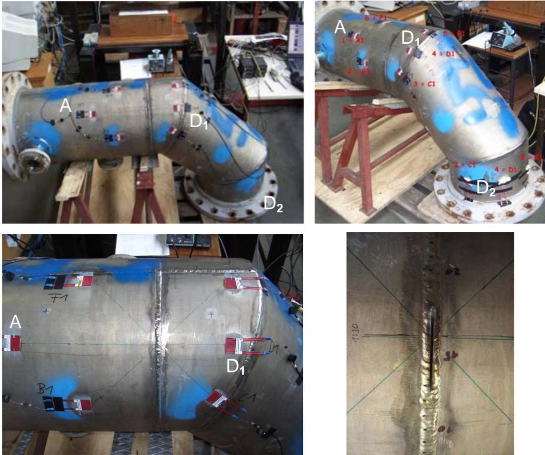
**Figure 10:** Titanium elbow (wall thickness = 6 mm) with notches artificially introduced into a weld seam. The notch depth was varied between 1 mm (first step) and 5.3 mm (last step). Due to the sawing the initial notch length of approx. 12 mm was also increased stepwise.
