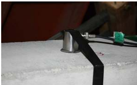
(a) sensor on the concrete
