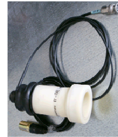
Electroacoustic sensor for pump rods
