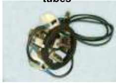
Electroacoustic sensor for pump-compressor tubes
