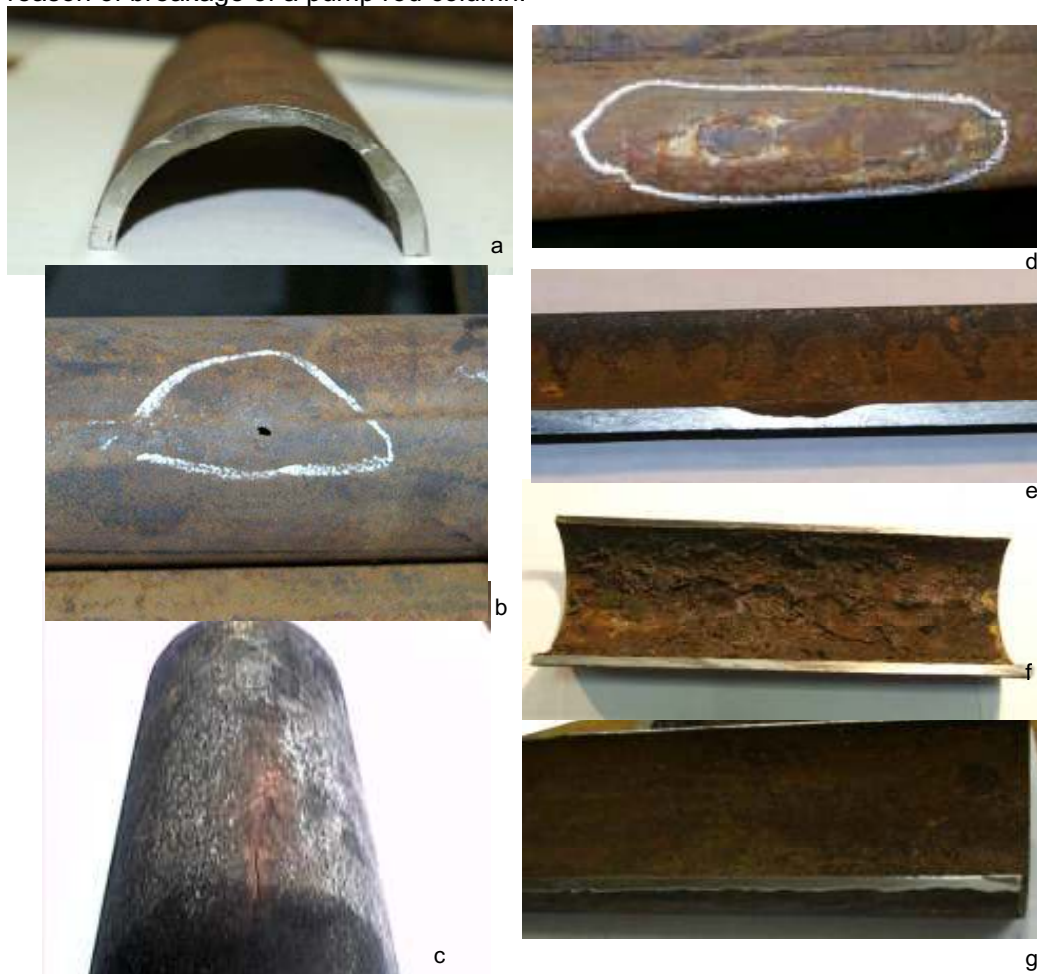
Fig.5. Snapshots of defects, detected in pump-compressor tubes: a - 2,3 mm wear of the inner tube surface caused by the coupling, b – through flaw, c - through crack, d – local corrosion of outer tube surface, e- 2,5 mm local corrosion of inner tube surface, f- extended corrosion of inner tube surface, g - extended corrosion of outer tube surface
