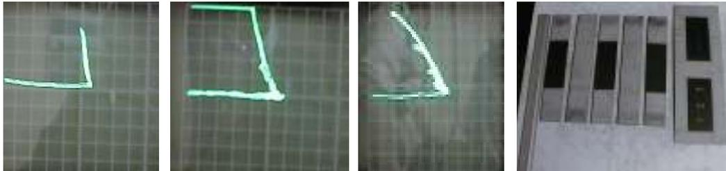
**Figure 1:** Waveform produced by the crack measured at the unpatched (1<sup>st</sup> photo) and the patched side (2<sup>nd</sup> photo) measured above the boron patch. Waveform produced by the three different cracks (0.5mm, 1mm and 2mm) above the boron patch of the calibration specimen (3<sup>rd</sup> photo). Specimens manufactured and calibration specimen (4<sup>th</sup> photo)
