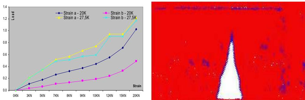
Figure 4: Debonding extension monitoring and final debonding area for specimens Type III.
