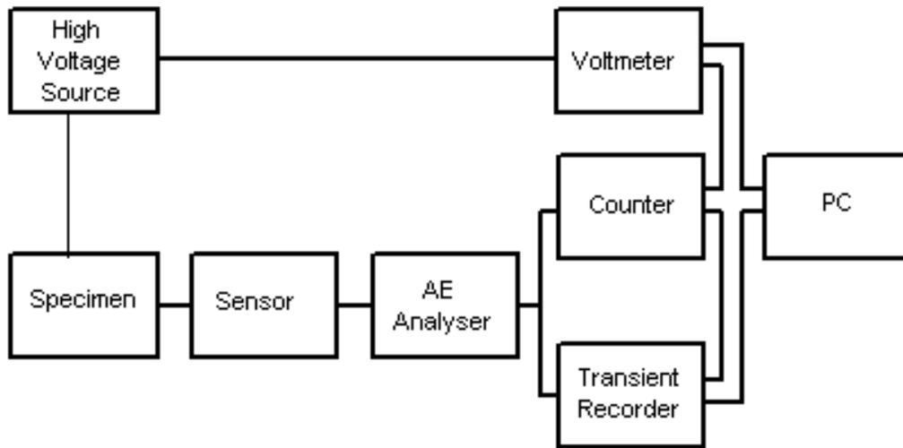
Fig. 1 Measuring apparatus diagram
