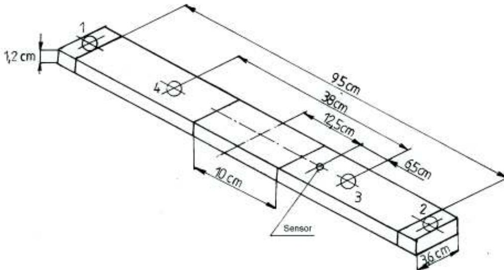
Fig. 2 Test specimen
