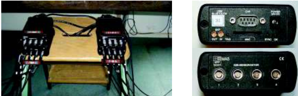
Figure 7: 4-channel sensor/actuator nodes for SHM of piping systems. The nodes can be combined to a multi-channel measuring system (16 channels in this case) that can be used for both active and passive monitoring. The present nodes are based on a CAN bus interface but wireless interfaces are also under development. Details of the hardware implementation can be found in [10].
