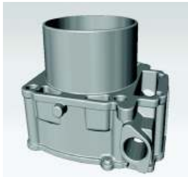
Fig. 1. 3D-CAD model of an Aluminium motorcycle engine cylinder
