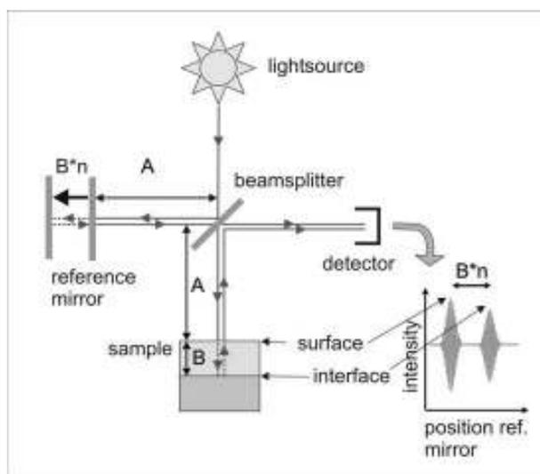
Figure 1: Schema of classical time-domain OCT setup using the Michelson interferometer geometry and a moveable reference mirror. A, B: optical path lengths, n: refractive index of sample layer.
