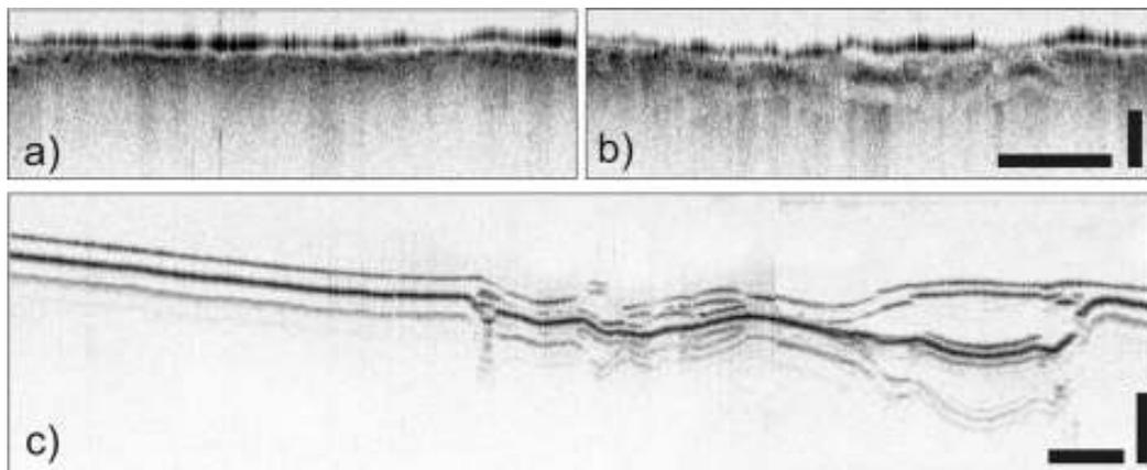
Figure 3: Cross-sectional images taken from layered polymer materials. a),b) powder coating on thermal treated wood, scale bars: 1mm (horizontal), 100  $\mu\text{m}$  (vertical); c) polymer coating on inside of a food container, scale bars: 1 mm (horizontal), 250  $\mu\text{m}$  (vertical).
