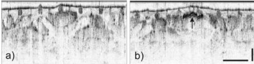
Figure 4: Cross-sectional images taken from a glass-fibre reinforced polymer composite: a) undamaged structure before loading procedure, b) defect region (arrow) after loading. Scale bars: 1 mm (horizontal), 100  $\mu$ m (vertical).
