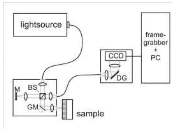
Figure 2: Schematic sketch of a spectral-domain OCT set-up. Abbreviations: beamsplitter (BS), mirror (M), Galvano-scanner mirror (GM), diffractive grating (DG), charge coupled device line camera (CCD).
