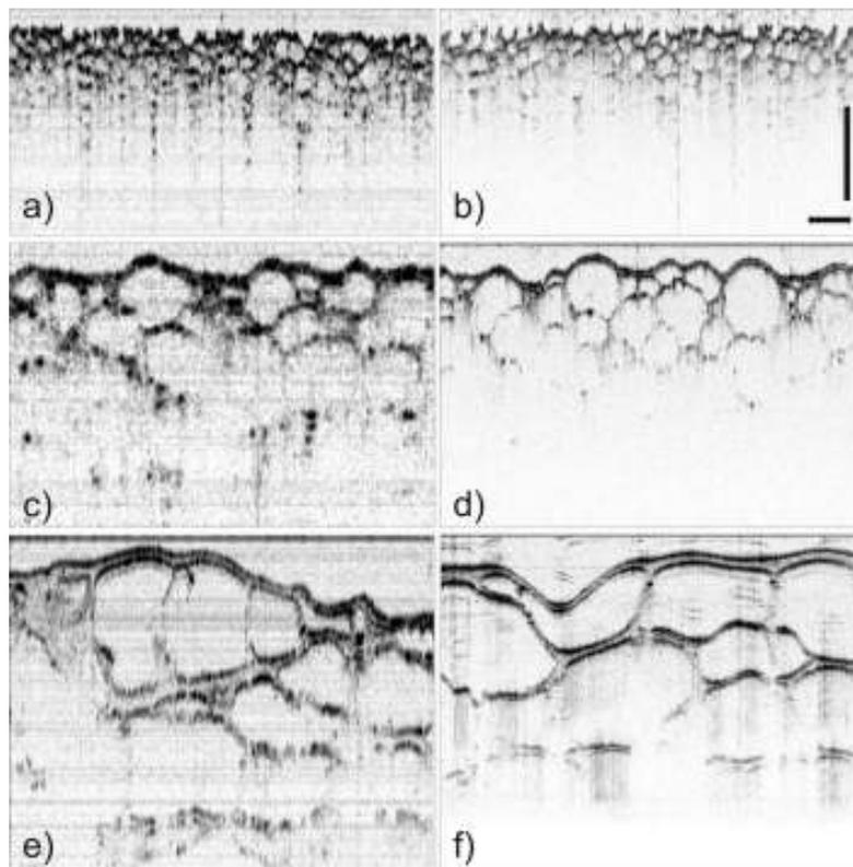
Figure 6: SD-OCT cross-sectional images taken from polymer foam samples with different pore sizes. a),c),e) images taken at a centre wavelength of 1550 nm, b),d),f) taken at 840 nm. Scale bars: 500  $\mu\text{m}$  (horizontal and vertical).
