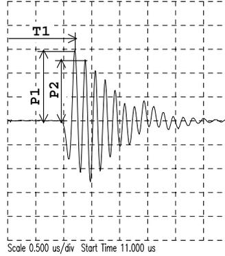
Fig. 3. Example of a receiving waveform using SH sensor.
