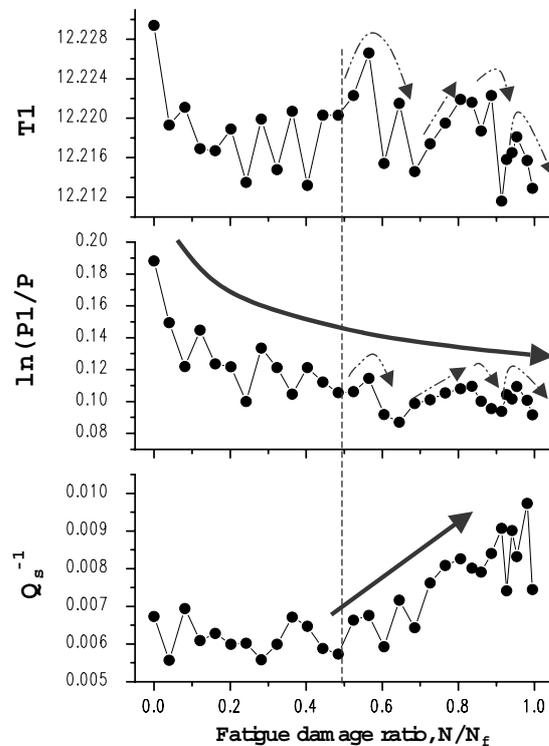
Fig. 4 Relationship for fatigue damage ratio of propagation time, logarithmic damping ratio and internal friction.
