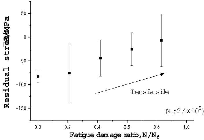
Fig. 6. Relationship between fatigue damage ratio and residual stress.
