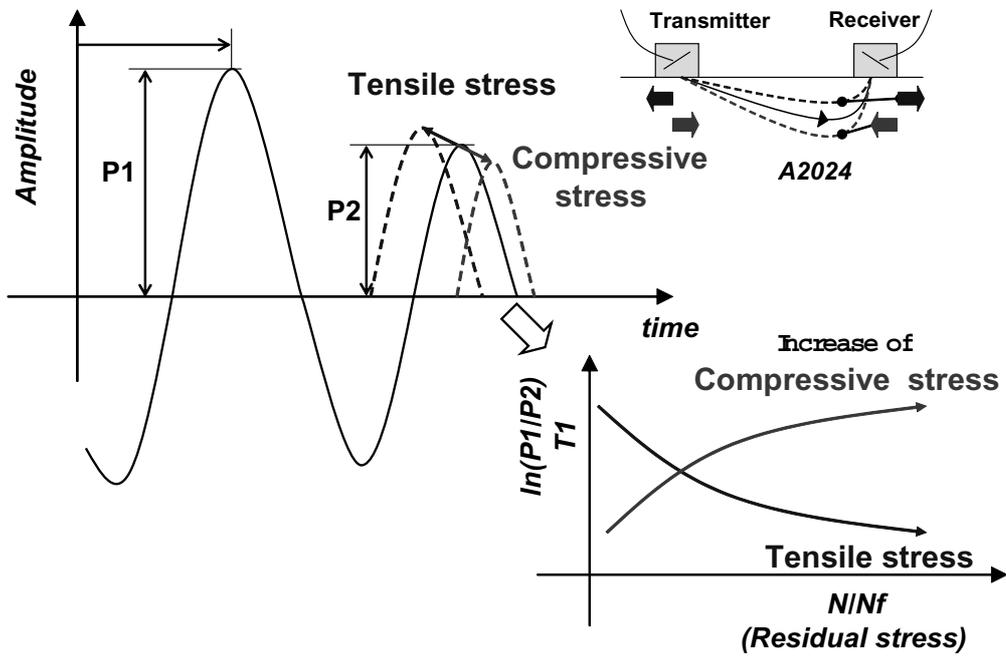
Fig.7. Relationship for the residual stress of logarithmic damping and propagation time.
