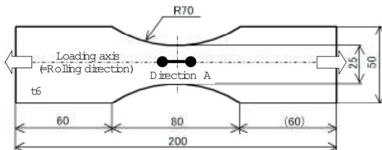
Fig. 1. Configuration of the tension test specimen (dimension in mm).
