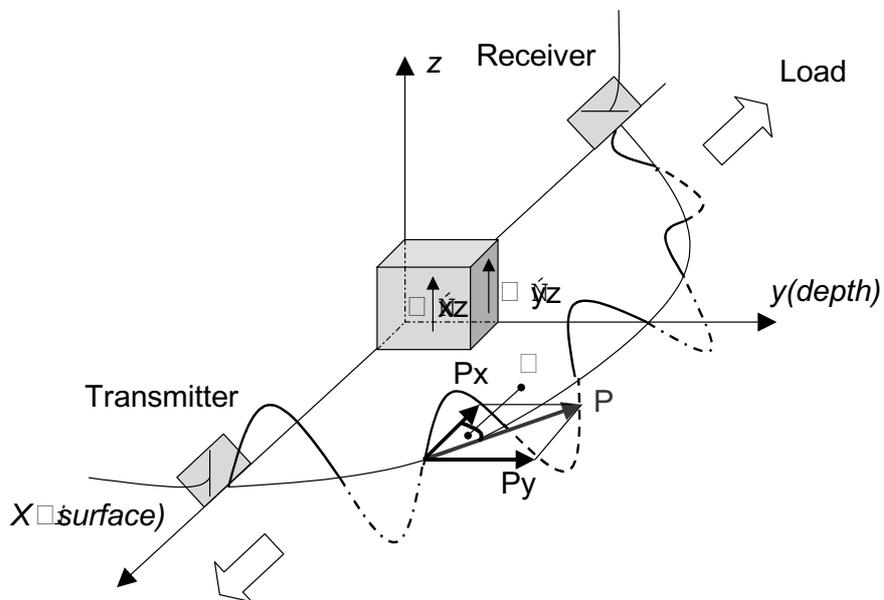
Fig.5 Energy flux of SH wave.
