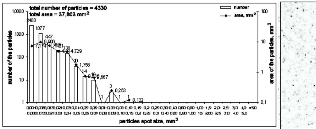
c) the print of the conventional offset printing used for recycling
