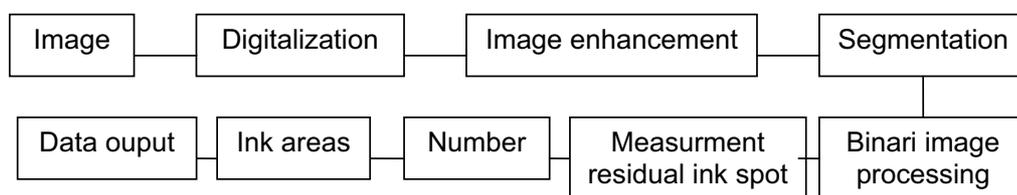
Figure 1: Dirt specks image analysis procedure
