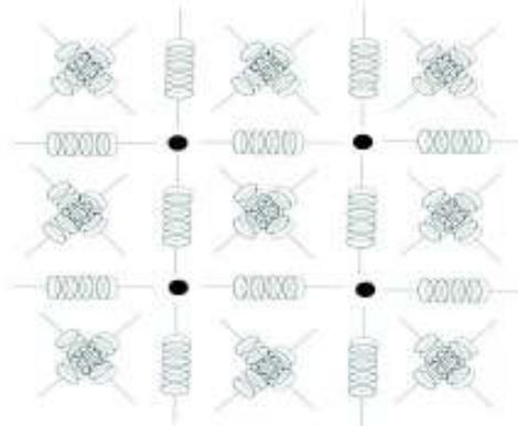
*Figure 1: Connections between nearby mass points of the numerical model*
