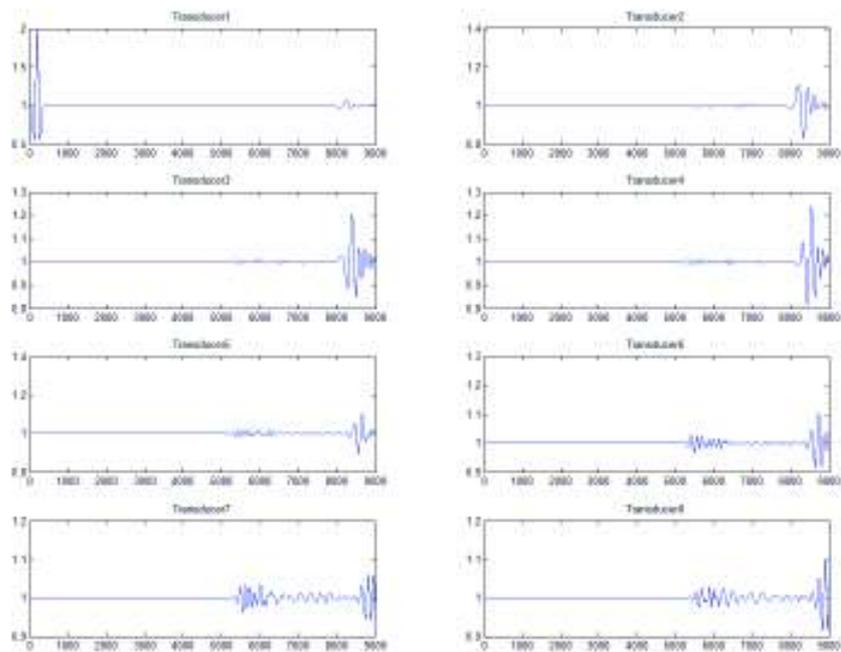
Figure 4: Simulation 2, test 1 (sending is transducer 1), recorded signals
