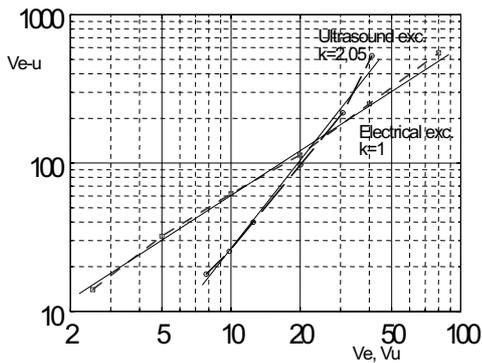
Fig. 8 Intermodulation component  $V_{E-U}$  vs. excitation signals  $V_E$  and  $V_U$
