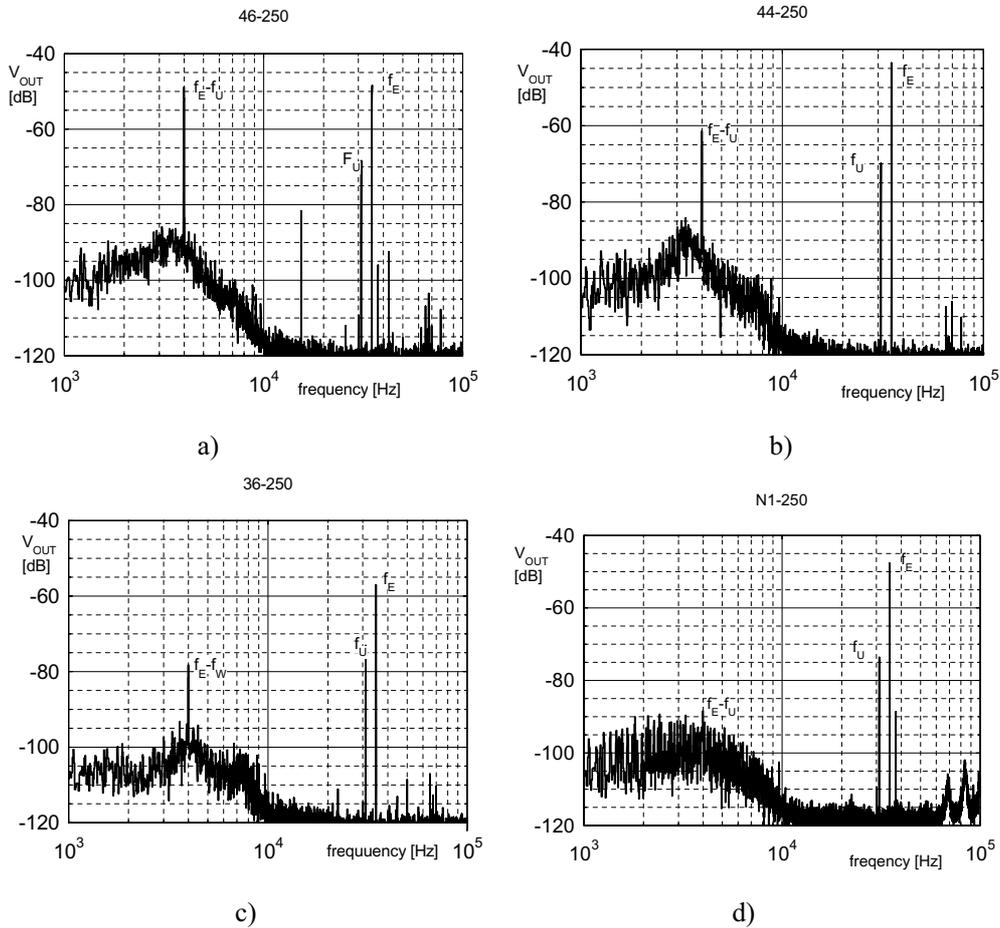
Fig. 9. Spectrum of measured signal for various samples: a-c) samples with cracks, sample without cracks.
