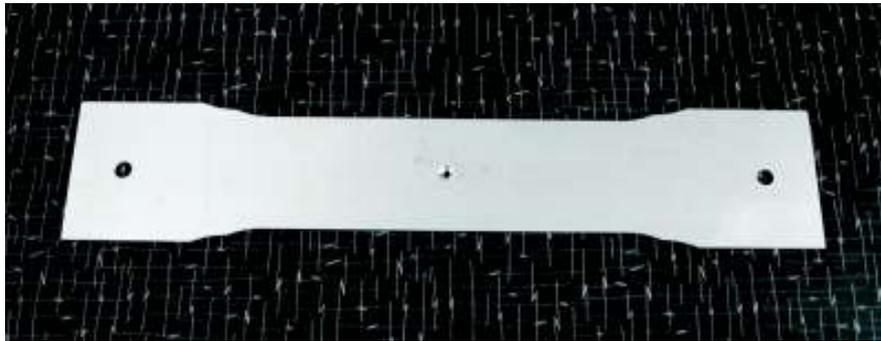
Fig. 7 The sample of a dural flat beam
