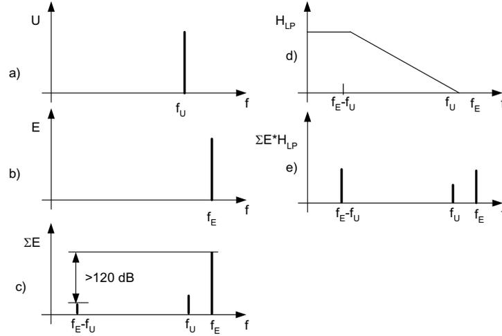
Fig. 2. Frequency spectrum of signals used by the parametric electro - ultrasonic spectroscopy: a) ultrasonic signal, b) electrical signal, c) resultant signal, d) frequency response of LP filter, e) filtered resultant signal with the lowered dynamic range
