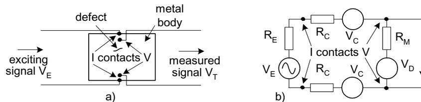
Fig. 5. Testing variant with current and voltage contacts and electrical substitution diagram: a) realization, b) electrical substitution diagram
