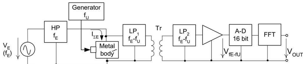
Fig. 6 Improved system of nonlinear ultrasonic-electrical spectroscopy
