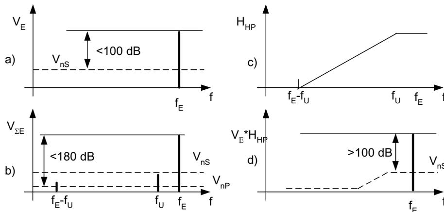
Fig. 3. Spectrum of signals and noise relations of the electrical source  $V_E$ : a) electrical exciting signal and noise, b) relations in the result signal in tested metal body, c) a frequency response of AC source HP filter, d) the exciting signal and noise after filtration
