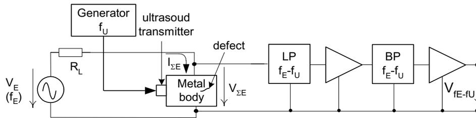
Fig. 1 Basic block diagram of the electro – ultrasonic spectroscopy
