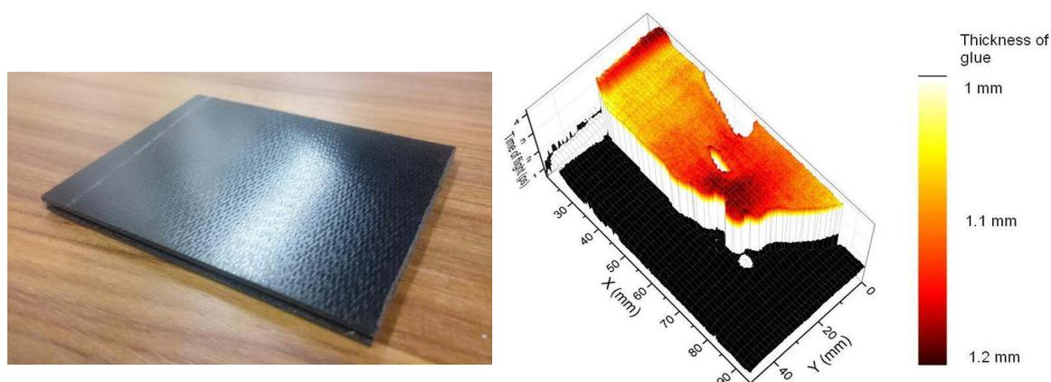
**Fig. 1.** Left: photo of two plates of GFRP glued by methyl methacrylate. Right: precise 3D reconstruction of the profile of glue between the plates thanks to fast scanning with the technology STRIPP.
