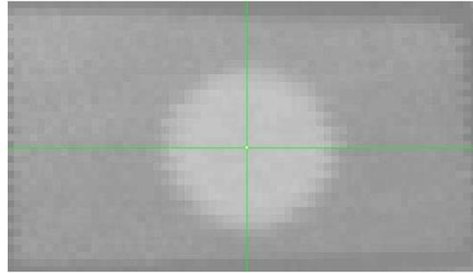
Fig. 10. C-Scan for area of GFRP sample with circular tefflon insert T4
