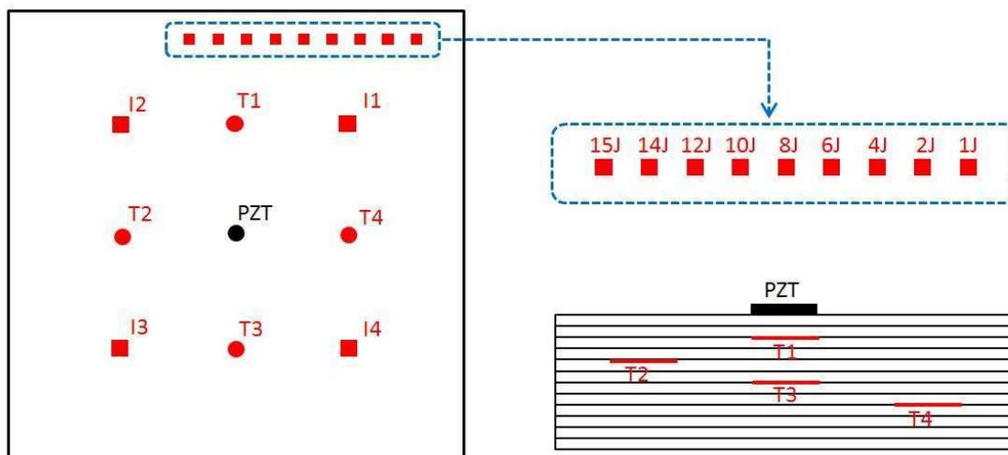
Fig. 2. Location of teflon inserts and impact damage
