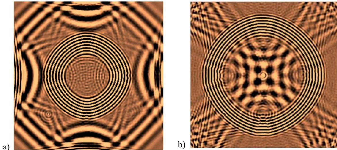
**Fig. 3.** Selected frames from animation of guided wave propagation in GFRP for excitation frequency 100 kHz: a, b) subsequent frames
