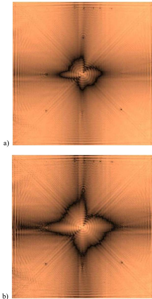
**Fig. 6.** WRMS energy map for excitation frequency 200 kHz: a)  $m=0.75$ , b)  $m=0.85$
