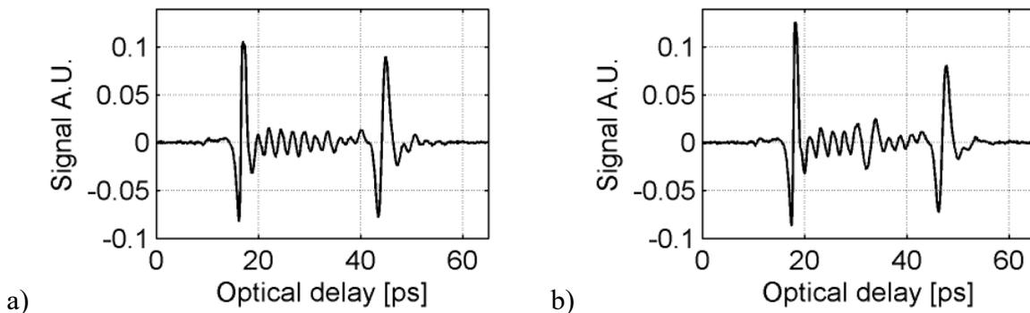
Fig. 7. THz Signals (A-scans) for GFRP sample: a) referential, b) material with teflon insert
