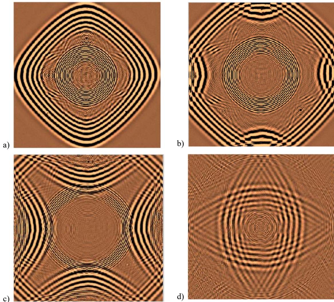
**Fig. 4.** Selected frames from animation of guided wave propagation in GFRP for excitation frequency 200 kHz: a-d) subsequent frames
