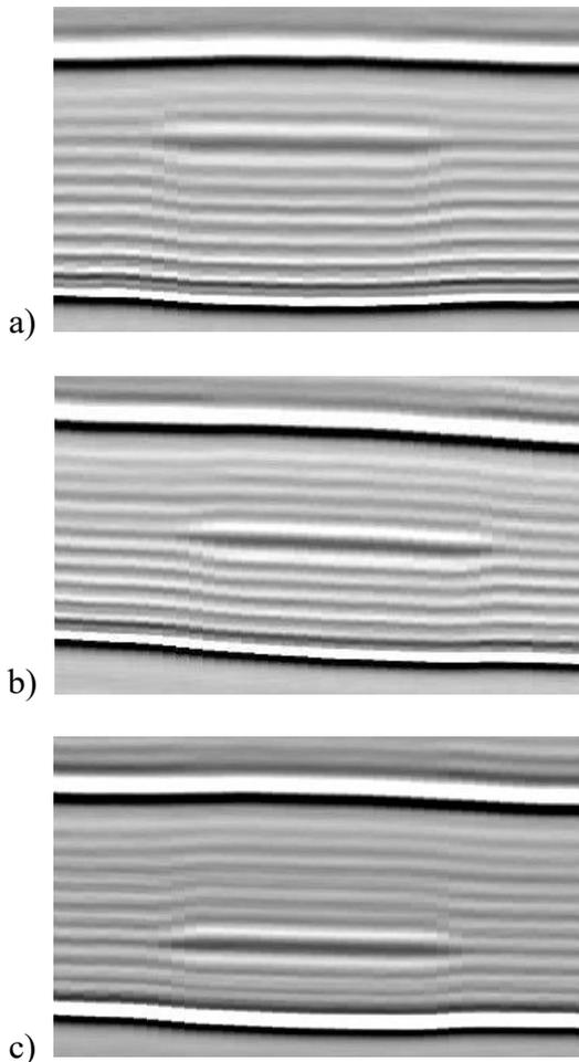
Fig. 8. B-scan for area of sample with circular teflon inserts: a) T2, b) T3, c) T4
