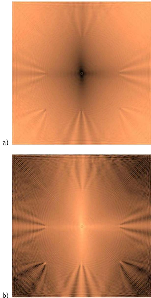
**Fig. 5.** WRMS energy map for excitation frequency 100 kHz: a)  $m=0.05$ , b)  $m=0.75$
