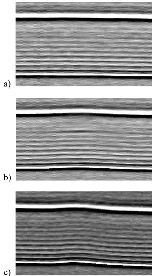
Fig. 9. B-scans for: a) referential area of sample, b) impact I3 – 10 J, c) impact I4 – 15 J
