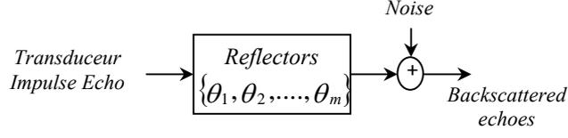
Figure 1. Parametric signal model for ultrasonic backscattered echoes.
