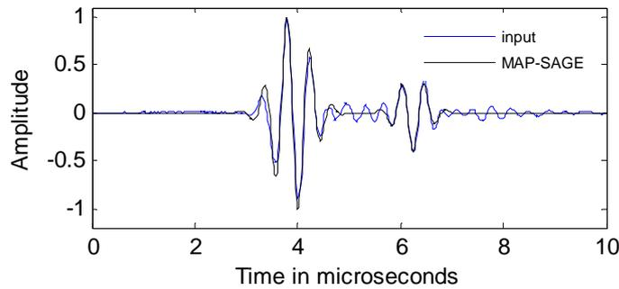
Figure 5: Signal in the undamaged zone (in blue line) and results obtained by MAP-SAGE in black line.
