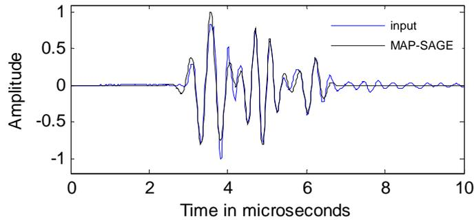
Figure 7: Signal in the damaged zone (in blue line) and results obtained by MAP-SAGE in black line.
