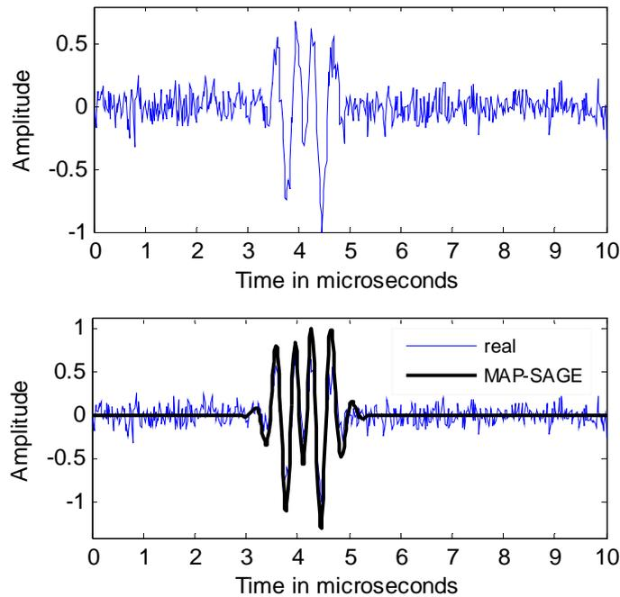
Figure 3: (a) Signal with two echoes with  $SNR=5dB$  separated by  $\Delta\tau=0.23\mu s$  (equivalent to  $0.32mm$ ), (b) Results obtained by MAP-SAGE in black line. Input signal in blue line.
