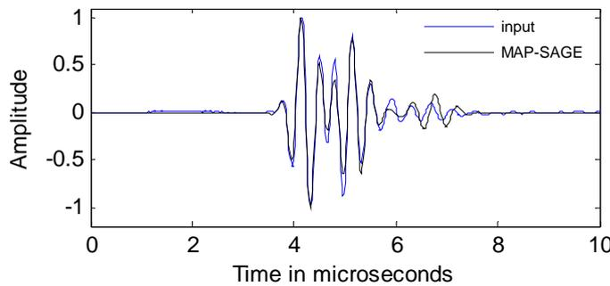
Figure 6: Signal in the damaged zone (in blue line) and results obtained by MAP-SAGE in black line.
