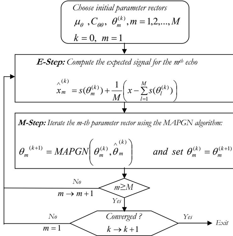
Figure 2: The flow diagram of the MAP-SAGE algorithm.
