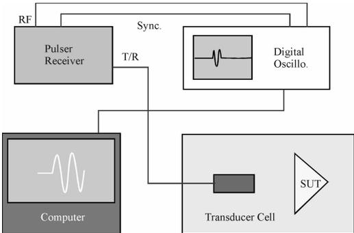
Figure1. Schematic diagram of the system measurement [1]
