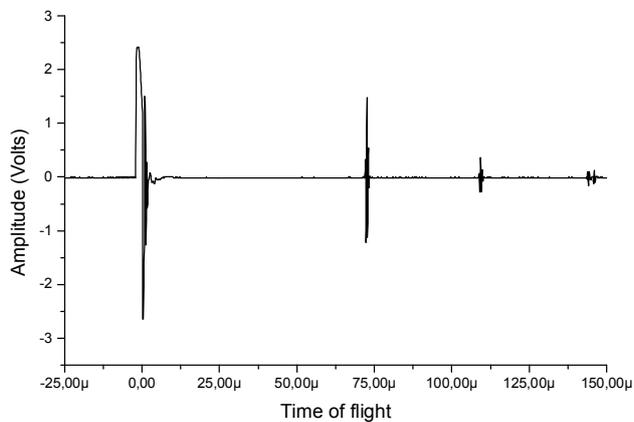
**Figure 8. Echo related to shear waves in Aluminium ( $t_t$ )**
