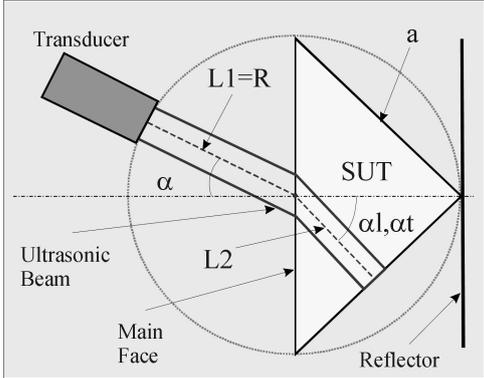
Figure2. Synoptic illustrating the technique of prism [2]
