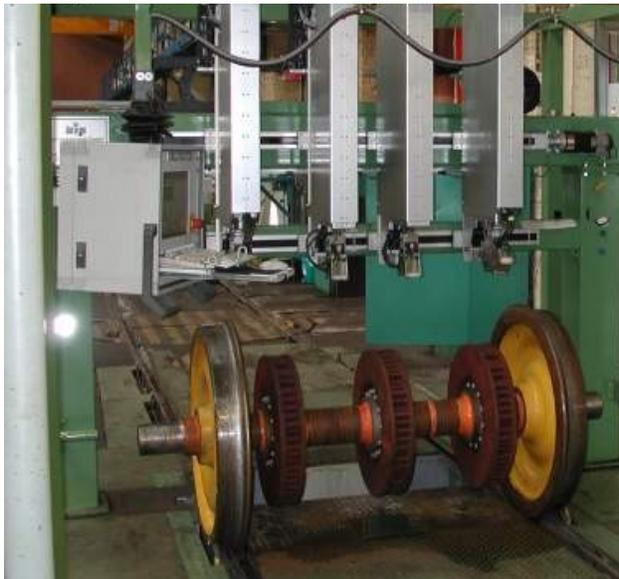
Fig. 7 Wheel set test system (DB)
