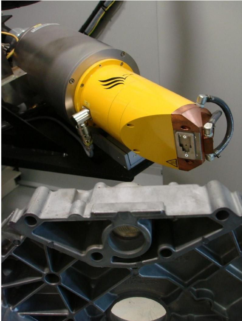
**Figure 4: The directional microfocus tube examining a large casting. The directional cone allows for higher energy X-rays to be generated.**
