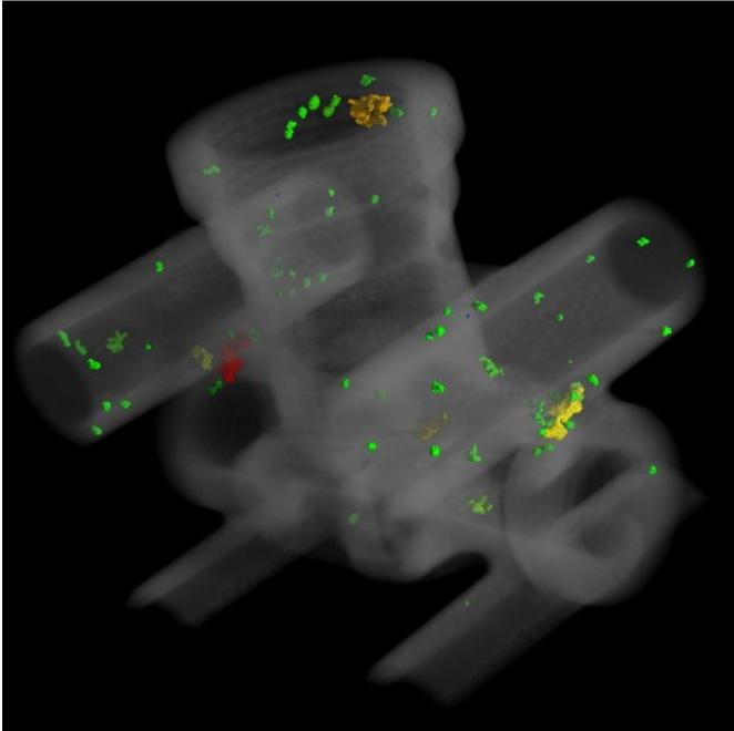
**Figure 5: Example of Pore Analysis using x|argos with image intensifier. Smaller Pores colored green, larger porosities yellow, orange and red.**
