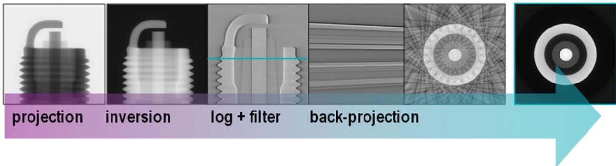
**Figure 3: Description of CT. The image stack is inverted and reconstructed using the geometry of the machine.**
