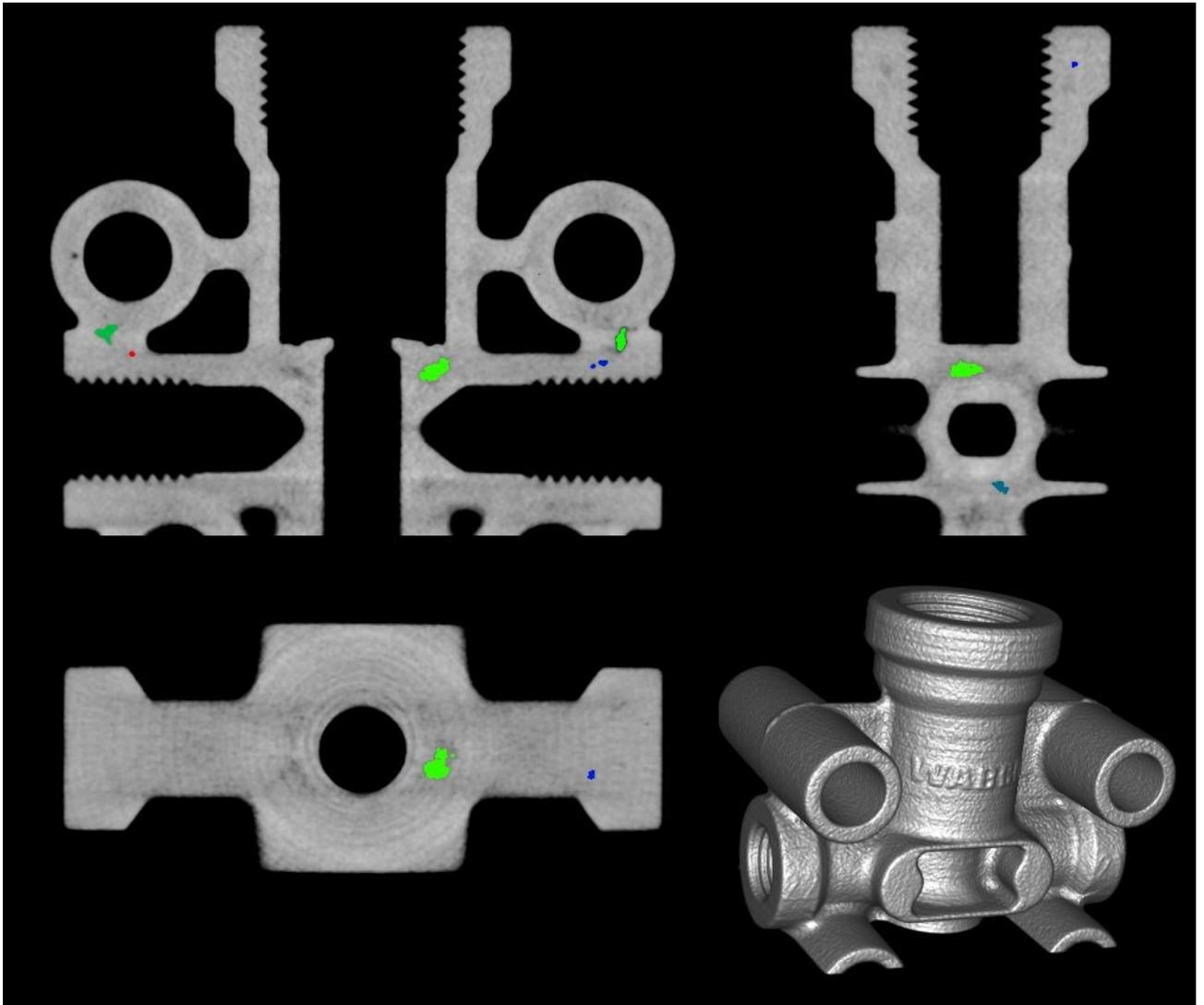
Figure 7: Four views of casting, examining in the xy, xz, and yz planes, as well as in 3D. Pores are highlighted using pseudocoloring.
