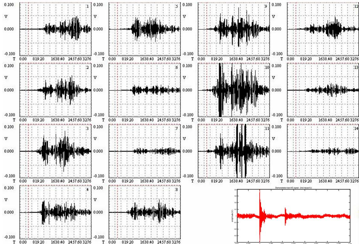
Fig. 3 Acoustic emission signal received from 14 different PZT patches, the signal in the right corner represents the signal received by optical fibre sensor.
