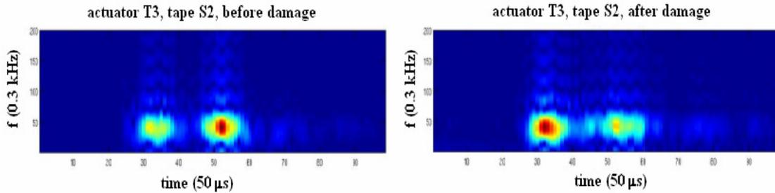
*Fig. 4 The time frequency images of the signals obtained using the optical fiber S2, and the actuator T3, before and after the impact was made. The frequency of the signal is 12 kHz, length of the signal array is  $N=25000$ , window size  $W=500$ ,  $I=250$ .*
