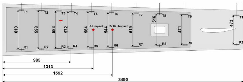
Fig. 2 Positions of transducers at the tail boom
