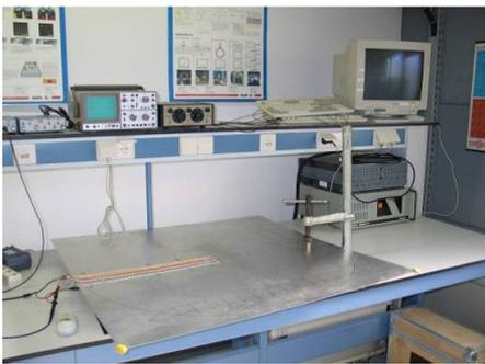
*Fig. 4 Mechanical application of non-destructive pseudo-defects on an aluminium plate*
