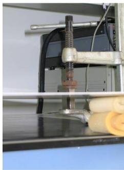
Fig. 4 shows the wired sensor array and the mechanical equipment used to establish a tough connection of two blocks with the aluminium plate. The blocks were iron cubes with a side length of 2 cm. It appeared that the pressure applied to the blocks had no influence on the reflection pattern once
