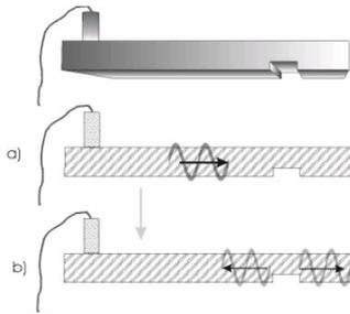
*Fig. 2 Interaction of a Lamb wave with an artificial notch reflection and attenuated transmission*
