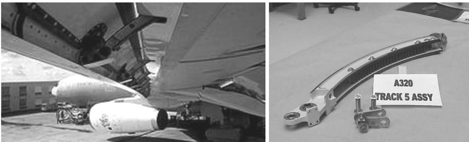
Figure 1 Slat tracks (Left side: positions in airplane wing – Right side: dismantled)
