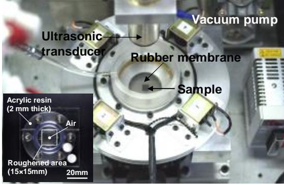
Figure 2: Details of dry ultrasonic transmission unit
