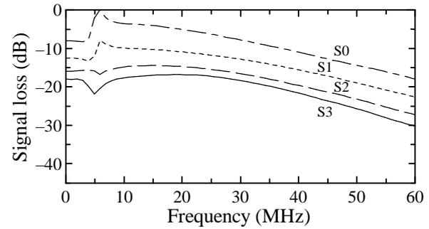
Figure 5: Relationships between the total signal loss and frequency (R4 membrane)
