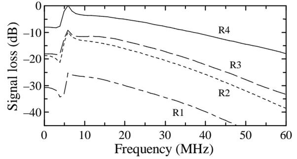
Figure 4: Relationships between the total signal loss and frequency (S0 sample)
