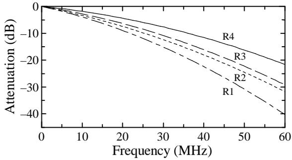
Figure 3: Ultrasonic attenuation in the used rubber membranes
