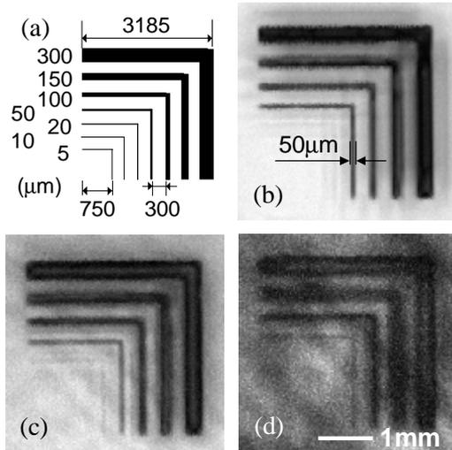
Figure 6: Fabricated nm gaps (a), and the acoustic images of Si-bonding sample obtained under the water immersion (b), R4-coupling (c) and R1-coupling (d)
