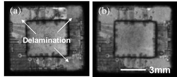
Figure 7: Acoustic images of a plastic package obtained under the water immersion (a) and R4-coupling (b)
