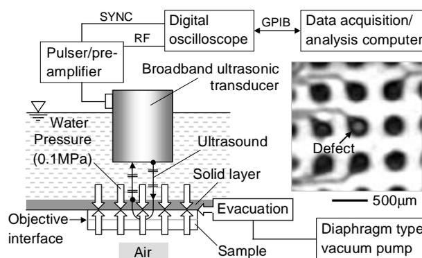
Figure 1: Schematic of dry-coupled acoustic microscopy technique
