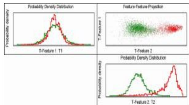
Figure 4: Separation of corrosion (red) and background noise (green) with the help of frequency domain based pattern recognition. The two features T1 and T2 have best separation power.
