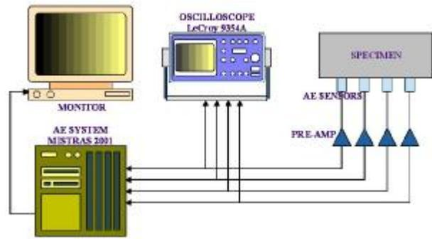
Fig. 4 acoustic emission data acquisition system
