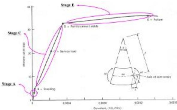
Fig. 1. Moment curvature diagram of RC beam
