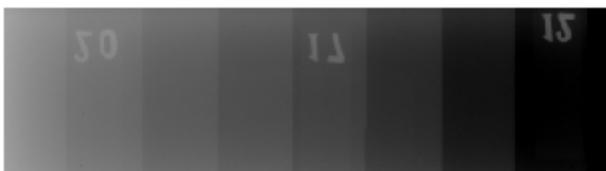
Figure 6: DR image of a step wedge with thickness ranging from 2-20mm
