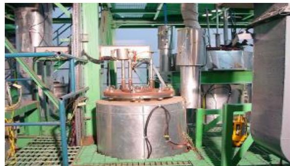
Figure 6: Sodium test vessel used for studying the influence of sodium in defects in steam generator tubes on remote field eddy current signals.
