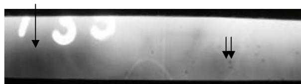
Figure 2 Concavity (arrow) and porosities (double arrow) of the order of 50 microns observed in one of a TTS weld Joint
