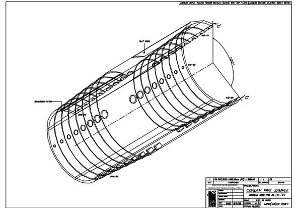
Fig.3 : The engineering design of artificial defects on pipe reference block.
