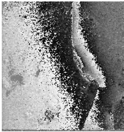
b) Shearogram made with thermal load
