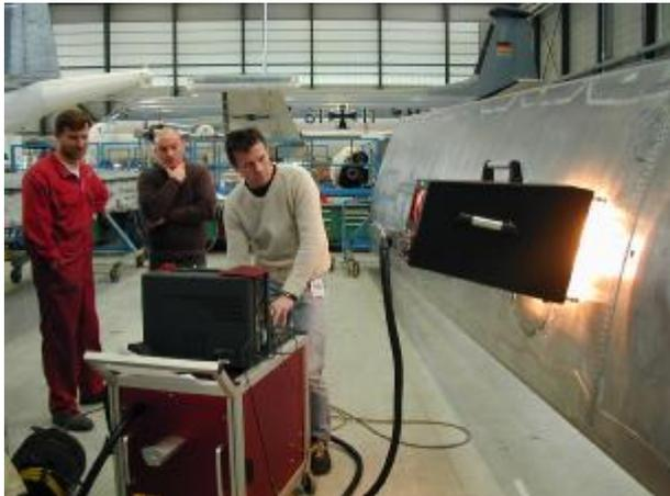
Fig.8: *Shearographic head-box applied on an aircraft wing.*
