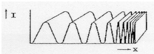
Graph 1: sinusoidal intensity distribution with increasing spatial frequency
