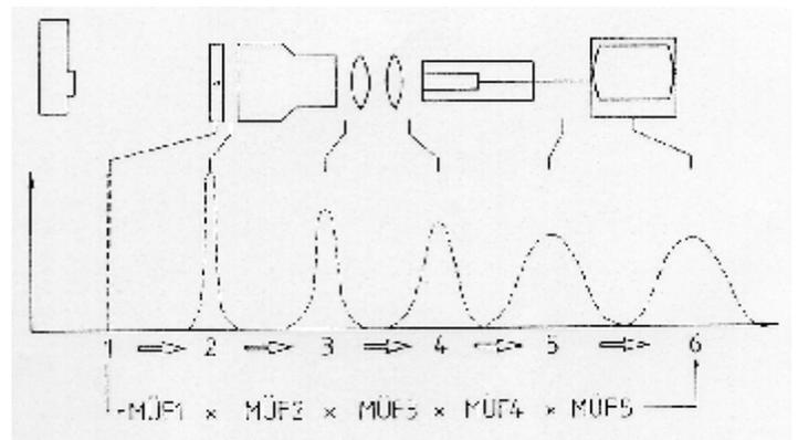
Fig.6: schematic diagram of the optical imaging process
