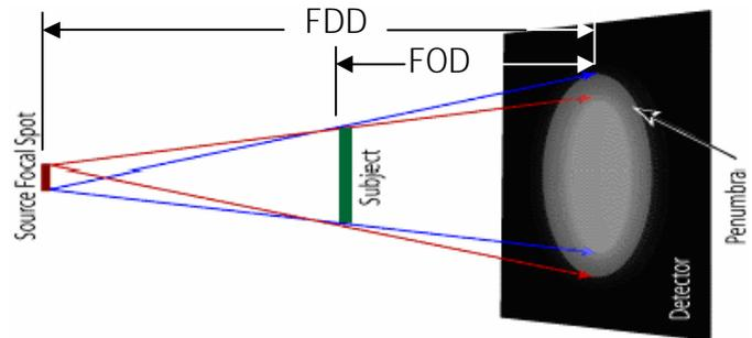
Fig. 2: real imaging geometry
