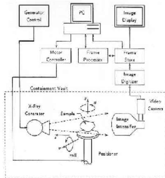
Workflow 1: radioscopy system set-up and imaging system
