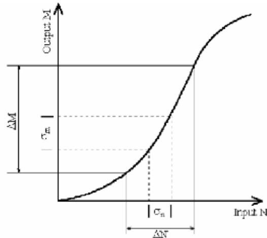
Graph 5: Signal to noise ratio for a given spatial frequency
