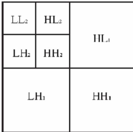
Figure 3: Subbands of the 2-D wavelet transform
