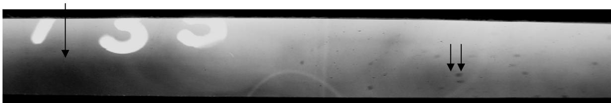
Figure 2: Uneven density variations introduced because of the varying beam angle. Note the density variations along and across the weld region.
