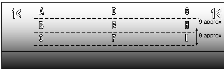
Figure 4: Typical locations on the radiographic films for density measurements.
