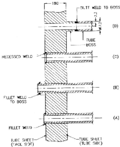
Figure 1: Typical joint configurations of tube to tubesheet welds
