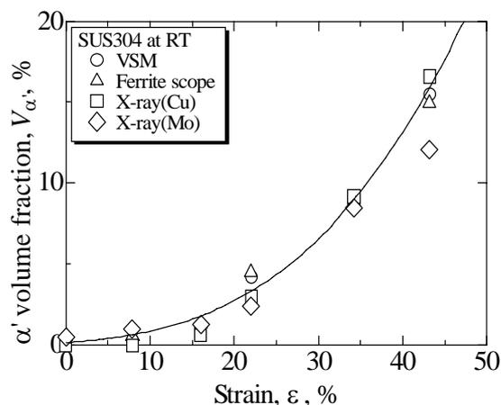
Figure 3: Plots of  $\alpha'$  volume fraction  $V_{\alpha'}$  vs. applied nominal tensile strain  $\varepsilon$  in SUS 304 stainless steel at RT obtained by different measurement methods.
