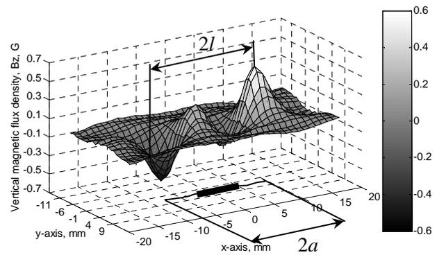
Figure 9: 3-D distribution of the vertical magnetic flux density  $B_z$  above a fatigue crack of  $2a=14.4$  mm at  $K_{max}=36.7$   $\text{MPa}\sqrt{\text{m}}$  for  $R=0.4$  in a SUS 304 steel plate specimen magnetized in the  $x$ -axis direction.
