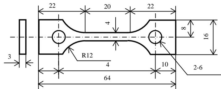
Figure 1: Geometry of tensile specimens (unit: mm).
