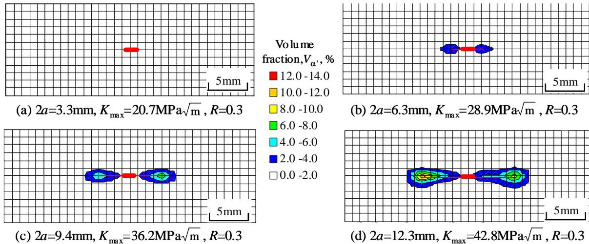
Figure 6: Evolution of the spatial distribution of  $\alpha'$  volume fraction around a through-thickness fatigue crack in SUS 304 steel measured by ferrite scope where  $2a$  is fatigue crack length,  $K_{\max}$  the applied maximum stress intensity factor and  $R$  the stress ratio.
