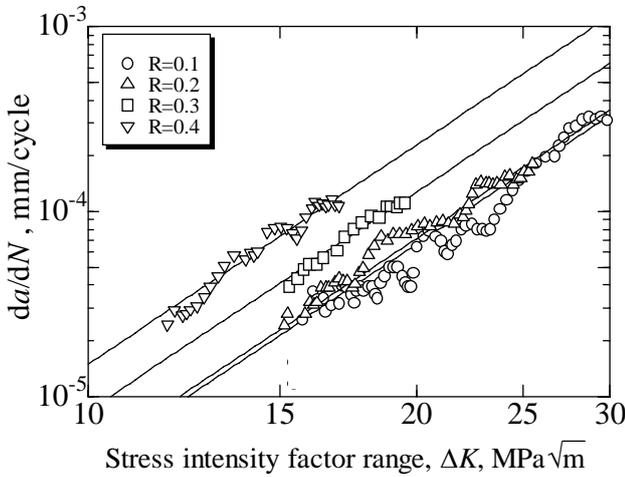
Figure 5: Comparison of fatigue crack growth behavior in SUS304 steel obtained for different values of the  $R$  ratio.
