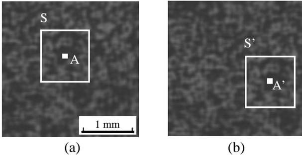
Figure 7: Random speckle pattern on the surface of a specimen.
