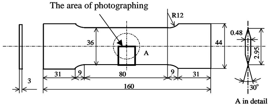
Figure 4: Geometry of through-thickness cracked specimen (Unit: mm).
