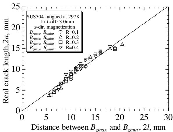
Figure 10: Real crack length  $2a$  as a function of the distance  $2l$  between the maximum and minimum peaks of the vertical leakage magnetic flux density distribution  $B_z$  above fatigue cracks in SUS304 plates.
