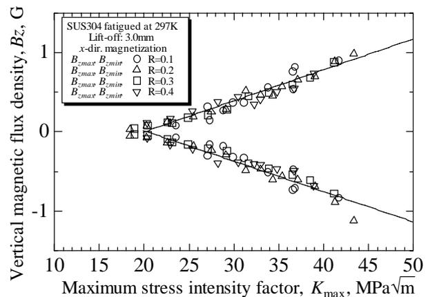
Figure 11: Maximum peak value  $B_{zmax}$  and minimum peak value  $B_{zmin}$  of vertical leakage magnetic flux density  $B_z$  vs. applied maximum stress intensity factor  $K_{max}$  relations.
