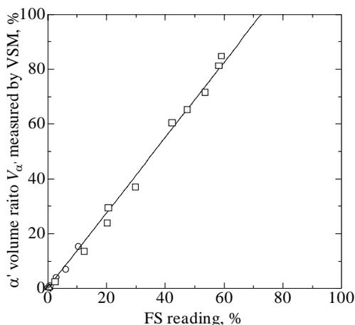
Figure 2: Calibration curve for for determining values of  $\alpha'$  volume fraction  $V_{\alpha'}$  by ferrite scope.
