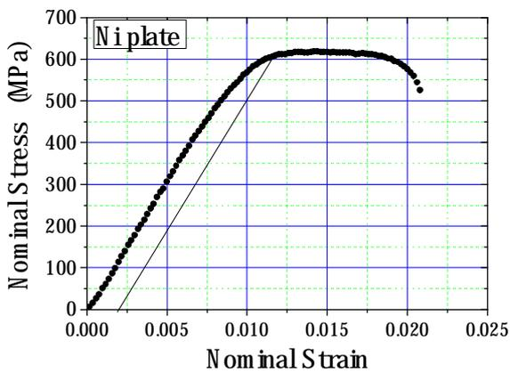
Figure 2: A result of a tension test for a rolled nickel plate.
