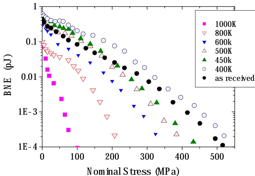
Figure 7: *Stress dependence of the Barkhausen noise energy (BNE) for nickel plates annealed at different temperatures.*
