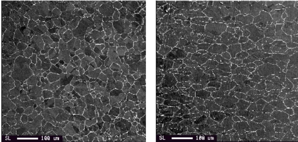
Figure 11: *Surface images of the nickel plate annealed at 1000 K before tension test (left) and after (right).*
