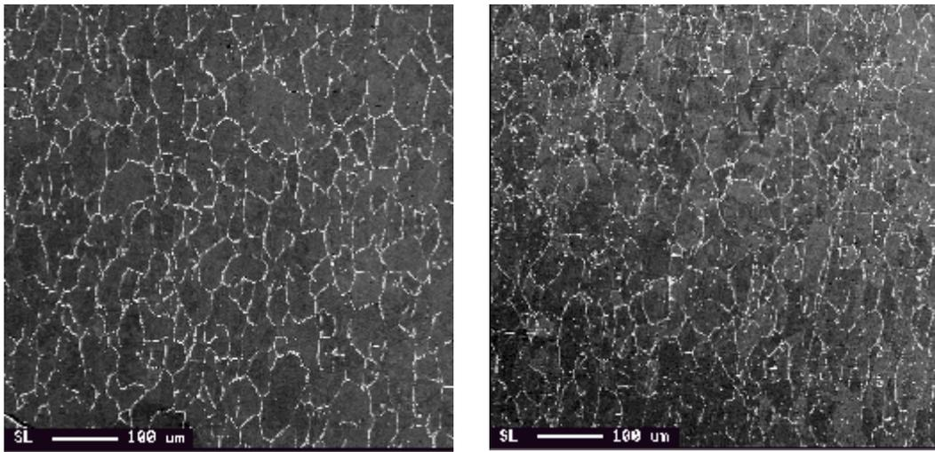
Figure 9: *Surface images of the nickel plate annealed at 400 K before tension test (left) and after (right).*
