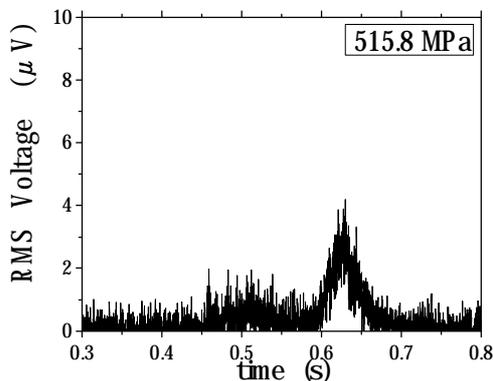
Figure 4: Rms Barkhausen noise profiles at various tensile stresses for the nickel plate.
