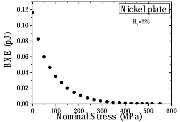
Figure 5: BNE versus nominal stress for a rolled nickel plate (see text).
