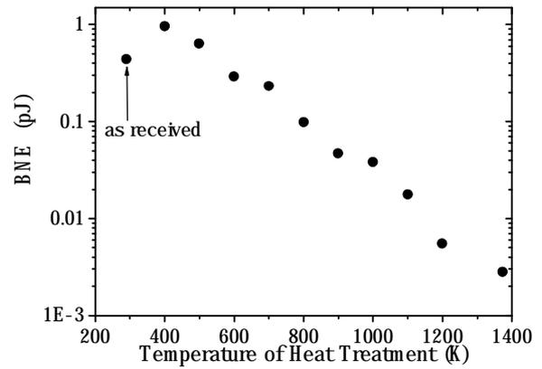
Figure 6: *BNE of annealed nickel plate as a function of temperature of annealing.*
