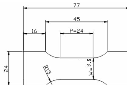
Figure 1: *The shape and size of a test piece.*
