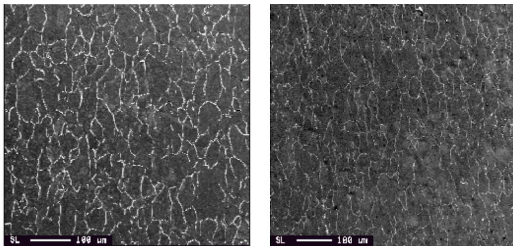
Figure 10: *Surface images of the nickel plate annealed at 600 K before tension test (left) and after (right).*
