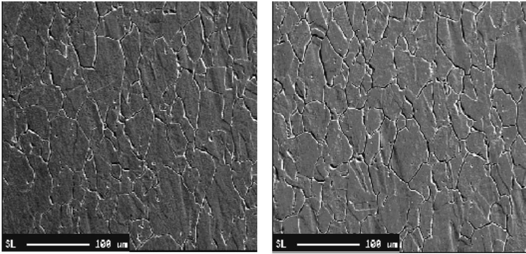
Figure 8: *Surface images of the rolled nickel plate as received before tension test (left) and after (right).*
