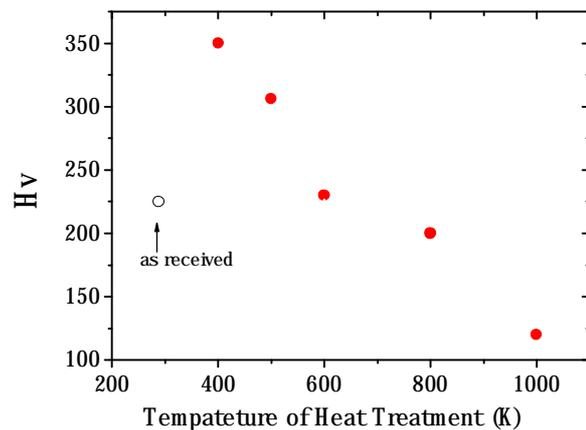
Figure 6: Vickers hardness of annealed nickel plate.
