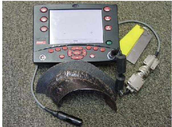
Absolute for Coating Thickness assessment Bridge / Differential for the detection of defects.
