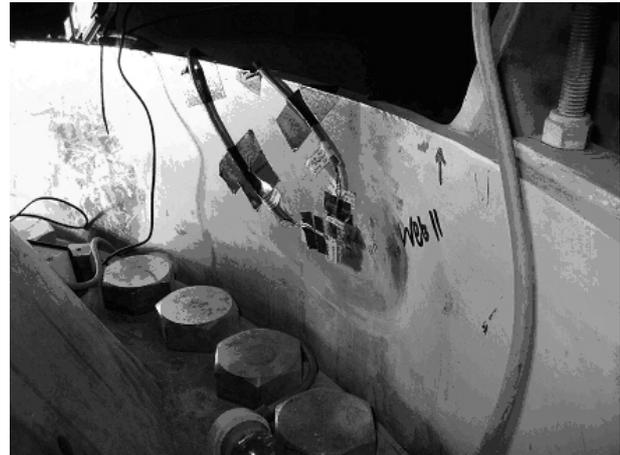
Figure 1: Skirt gauges 3 and 4 near web 11. Gauge 4 is located 120 mm circumferentially from web 11, and 120 mm vertically down from the top surface of the skirt. Gauge 3 is located 10 mm below gauge 4.
