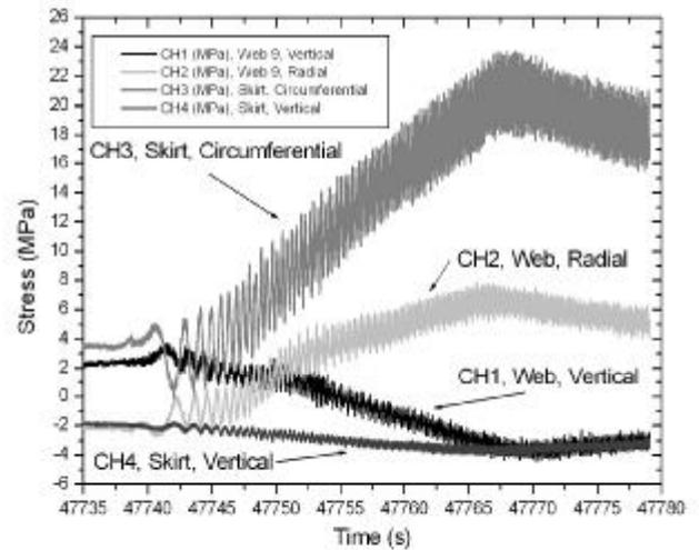
Figure 2. Warm rotor startup, 2.5 kV excitation.
