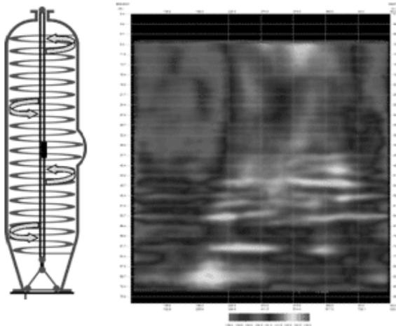
Figure 6: Coke drum spiral laser scanning system and 2d plot of inspection data.
