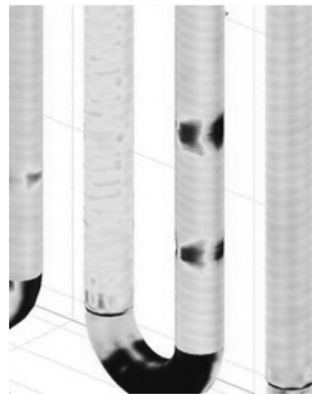
Figure 5: Typical graphical display of FTIS inspection data.
