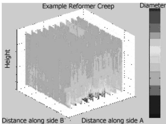
Figure 7: Typical LOTIS inspection results showing creep strain.
