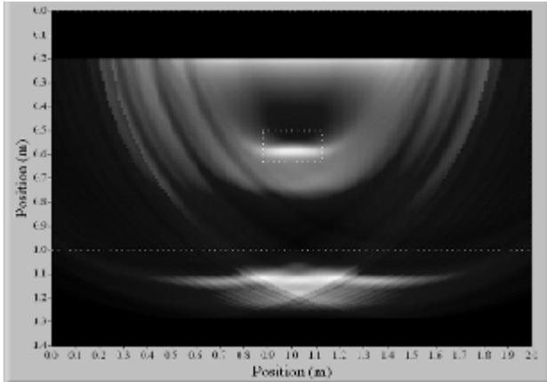
Fig. 9. Revised SAFT image generated from displacement responses of concrete specimen with wave velocity being 10% higher than actual value and single rectangular void bar.
