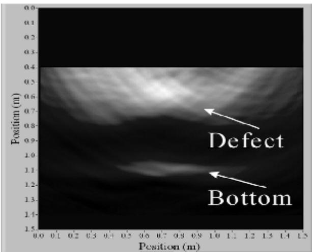
Fig. 16. Revised SAFT image generated from responses of experimental concrete specimen subjected to an impacting of 8mm steel ball.
