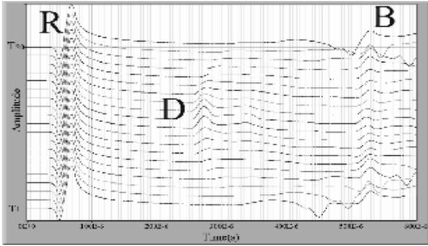
Fig. 3. B-scan displacement diagram of concrete specimen with single rectangular void bar in numerical simulation.
