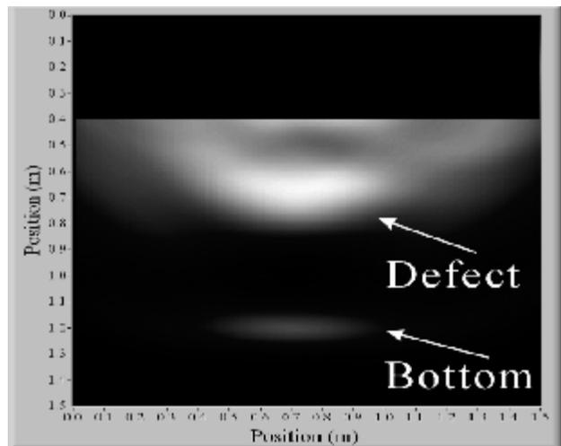
Fig. 14. Revised SAFT image generated from responses of experimental concrete specimen subjected to an impacting of 19mm steel ball.
