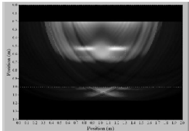
Fig. 8. Revised SAFT image generated from displacement responses of concrete specimen with two rectangular void bars.
