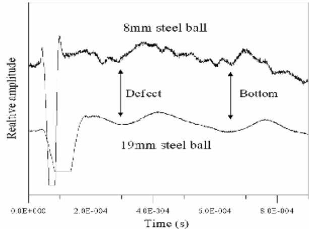
Fig. 17. Comparison of displacement responses of experimental concrete specimen subjected to the impacting of 19mm and an 8mm steel ball.
