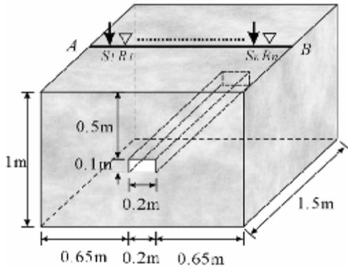
Fig. 12. Dimensions of concrete specimen with rectangular void bar for experimental study.
