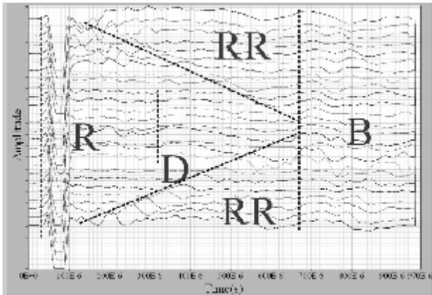
Fig. 15. B-scan displacement diagram of experimental concrete specimen subjected to an impacting of 8mm steel ball.
