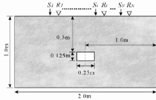
Fig. 2. Dimensions of concrete specimen with rectangular void bar for the study of numerical simulation.
