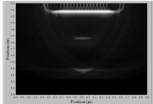
Fig. 4. Original SAFT image generated from displacement responses of concrete specimen with single rectangular void.
