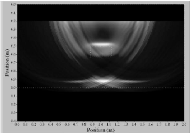
Fig. 10. Revised SAFT image generated from displacement responses of concrete specimen with wave velocity being 10% lower than actual value and single rectangular void bar.
