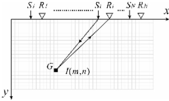
Fig. 1. Schematic showing the implementation of impact-and-receive operations and meshing of specimen for image processing with SAFT.
