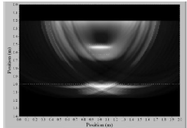
Fig. 5. Revised SAFT image generated from displacement responses of concrete specimen with single rectangular void bar.
