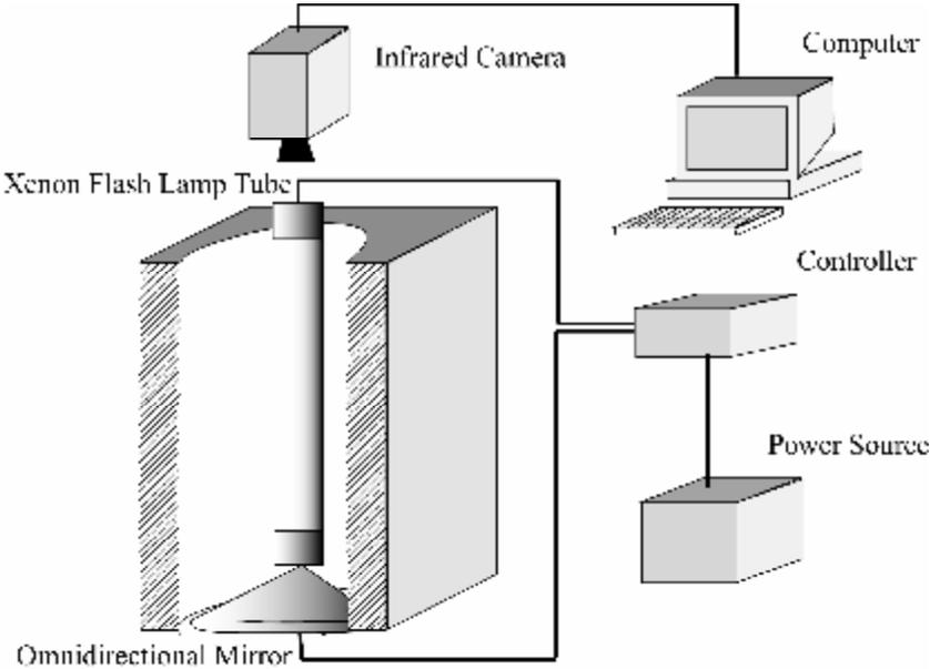
Figure 7: Schematic illustration and photograph of thermographic NDI system
