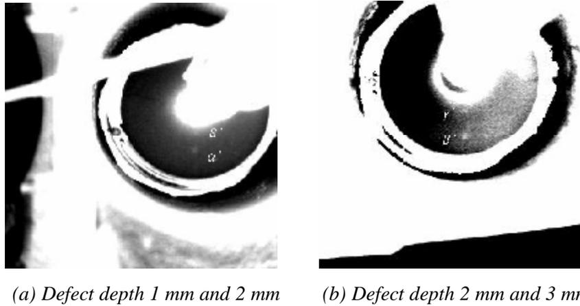
Figure 8: Thermal images of inner surface of cylinder reflected on omni-directional mirror
