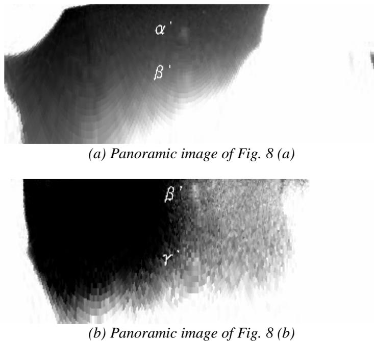
Figure 9: Panoramic image of inner surface of cylinder transferred from thermal images in Fig. 8.
