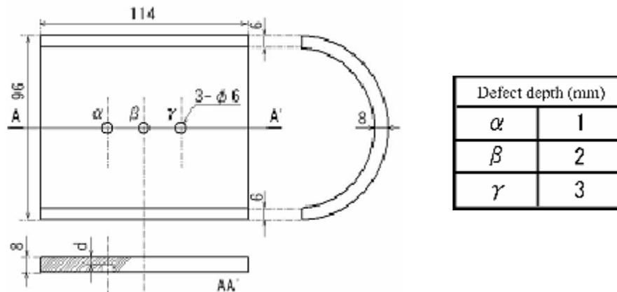
Figure 4: Configuration of employed half-cut cylinder specimen with flat-bottom hole defects
