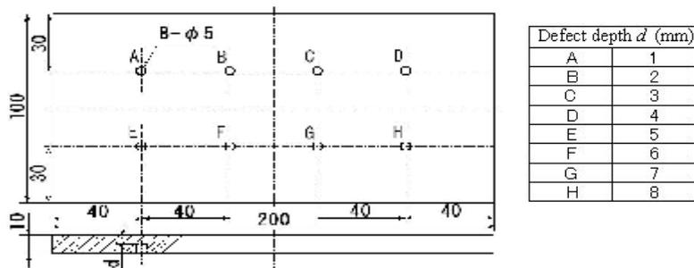
Figure 2: Plate specimen with flat-bottom hole defects
