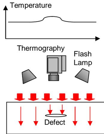
Figure 1: Schematic illustration of thermographic NDI
