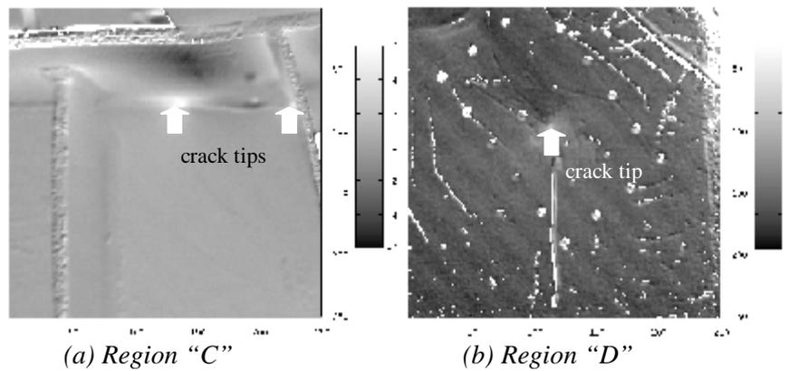
Figure 7: Results of crack detection in steel structure specimen.
