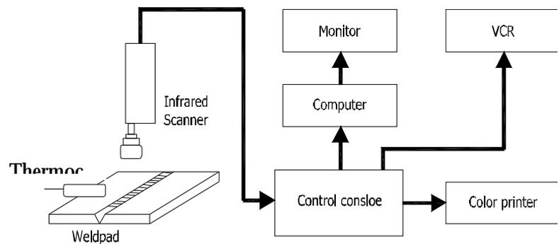
Figure 2: Schematic of the experimental set up for online weld monitoring studies
