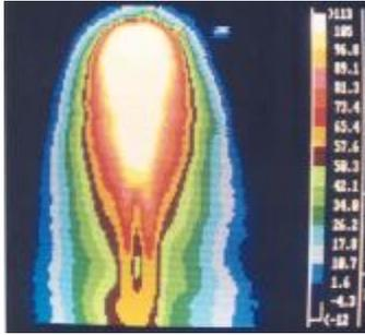
Figure 3: Isothermal profiles of lack of penetration formed during root pass
