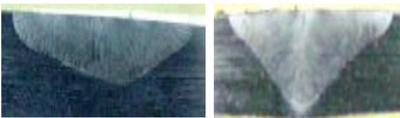
Figure 7: Cross section view of partial and full penetration weld.
