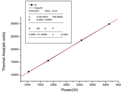
Figure 6: A plot of thermal area Vs input power of the welding machine
