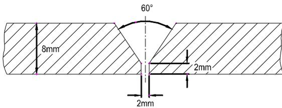
Figure 1: Typical weld joint design
