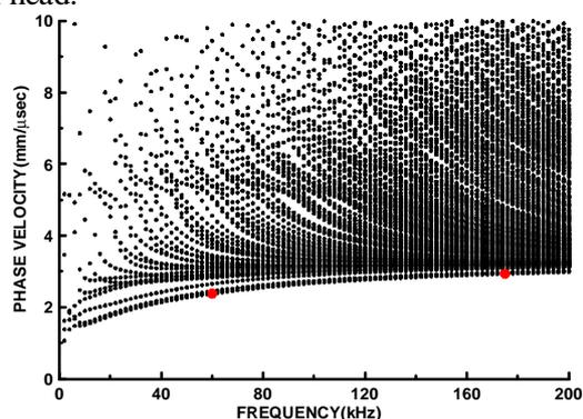
Figure 1 Phase Velocity dispersion curves of a rail
