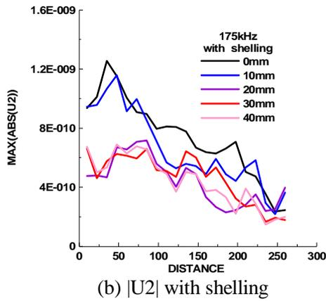
Figure 5 Absolute value of  $U_2$  of the transmitted wave at several points (175kHz)
