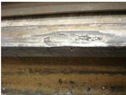
Figure 10 A Photograph of a hole in a rough rail
