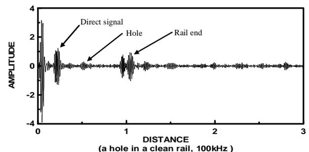
Figure 8 RF wave form of a reflected wave from a hole in a clean rail for a 100kHz
