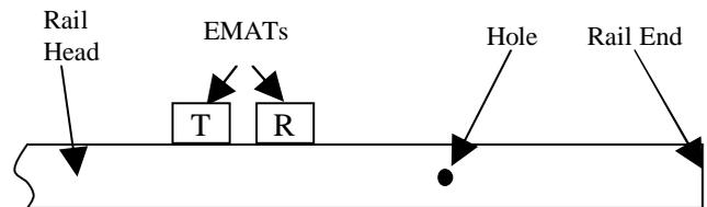
Figure 7 The position of a hole and EMATs
