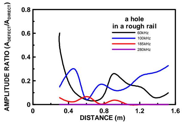
Figure 11 Amplitude ratio for a rail with a rough rail head surface and a hole showing that guided waves for 60kHz and 100kHz can find the hole, 185kHz is marginal, and the 280kHz guided wave cannot see the hole since a collection of small echoes from the rough surface does not allow any energy to reach the defect
