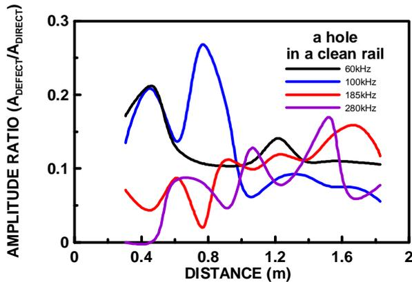
Figure 9 Amplitude ratio for a rail with a clean surface of a rail head and a hole showing that at a distance less than 1m, 60kHz and 100kHz guided waves have more potential for detecting the hole
