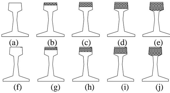
Figure 2 Cross-section of the rail with shelling and various defects ( (a):no defect, (b):10mm defect, (c):20mm defect, (d):30mm defect, (e):40mm defect, (f):shelling, (g):10mm defect with shelling, (h):20mm defect with shelling, (i):30mm defect with shelling, (j):40mm defect with shelling)
