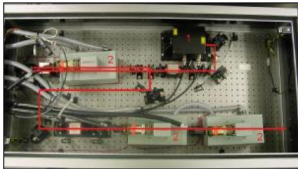
Fig.7: The Nd:YAG detection laser. The seed laser is marked with 1, the three amplifiers are marked with 2.
