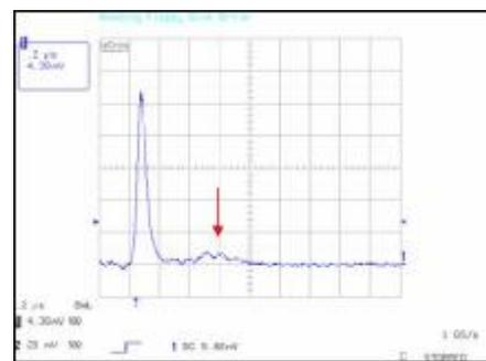
Fig.6: Modified TEA-CO<sub>2</sub>-laser pulse.
