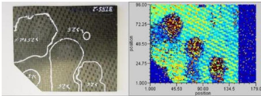
Fig.9a: Photo of the 4mm thick CFRP. Fig.9b: C-Scan obtained with laser ultrasound.
