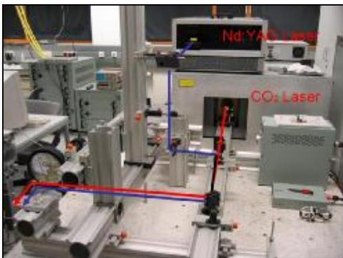
Fig.5: Beam propagation of the system (red line CO<sub>2</sub>-laser, blue line Nd:YAG laser).
