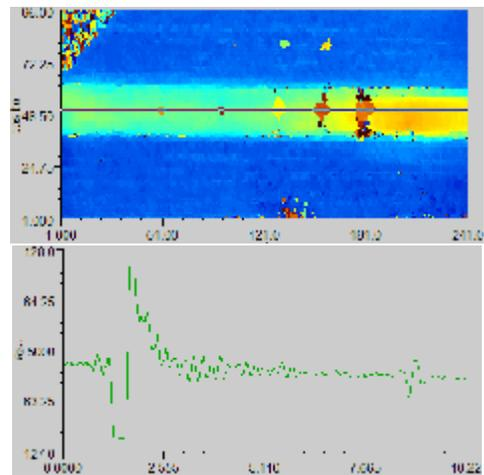
Fig.13: Time of flight scan with the corresponding A-Scan including the measuring window.
