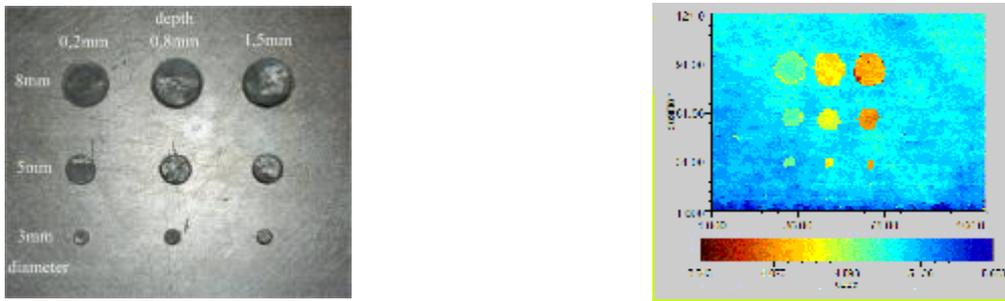
Fig.8: Test component with holes. Left: backside of the component. Right: time of flight scan with scale.
