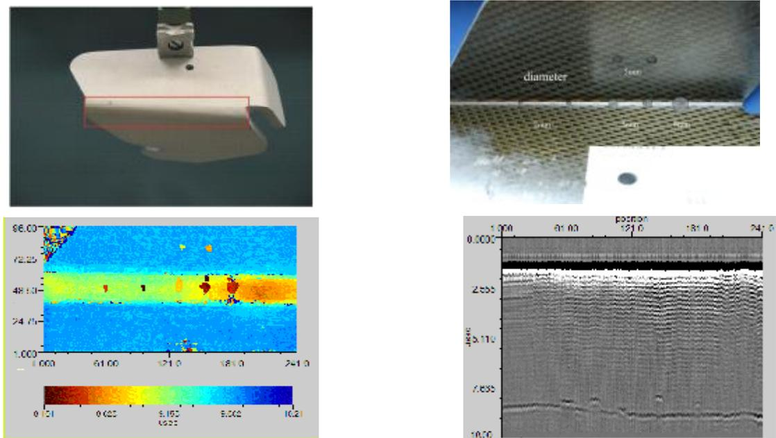
Fig.11: Top: View from the detection optics onto the shaped part. Top right: Rear side with inserted flaws. Bottom left: Time of flight C-scan. Bottom right: B-scan out of the area of curvature.
