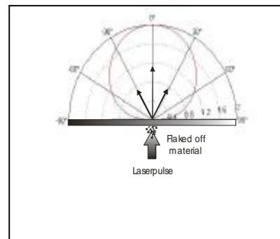
Fig.3: Ablative laser ultrasound generation: The recoil of the particles flaking off from the surface generates a longitudinal wave perpendicular to the surface.
