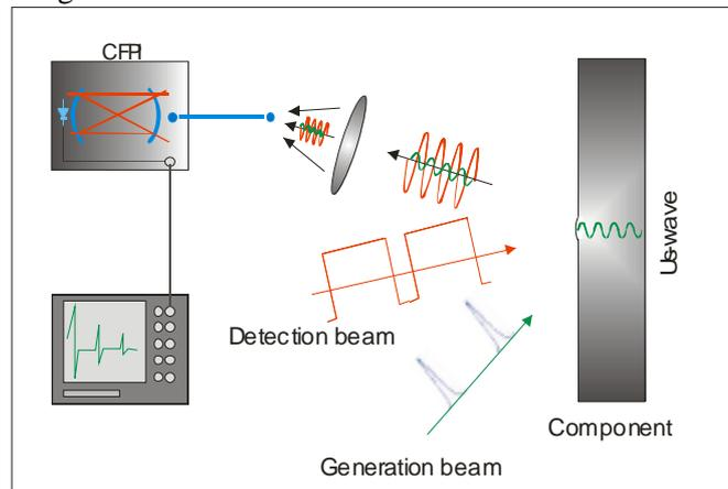
Fig.2: Principle of the laser ultrasound technique.
